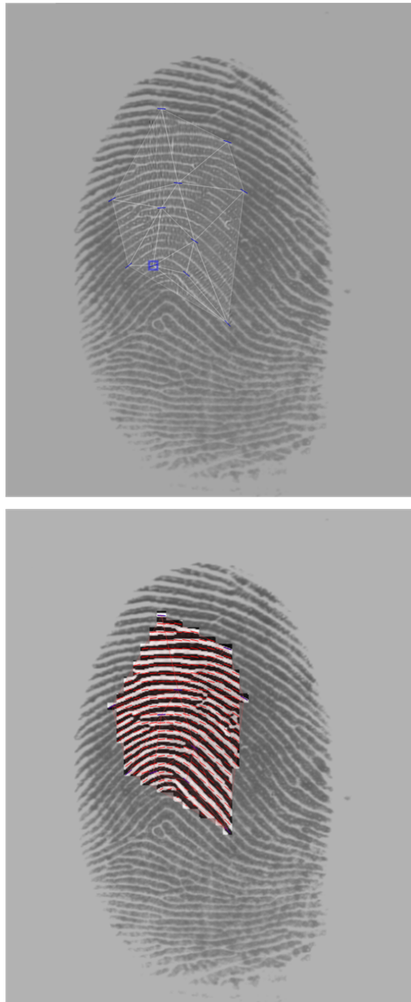
Figure 6.3: FOE Ground-truth markup. Example of ground-truth markup of a fingerprint that belongs to the FOE benchmark. Some local orientations are marked up by the user (vertices of triangles on the top image); others are interpolated by the software (bottom image).
