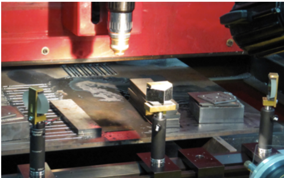
Fig. 13: Picture of the optical setup for multi-view high-speed imaging. (taken from Ref. 11)
