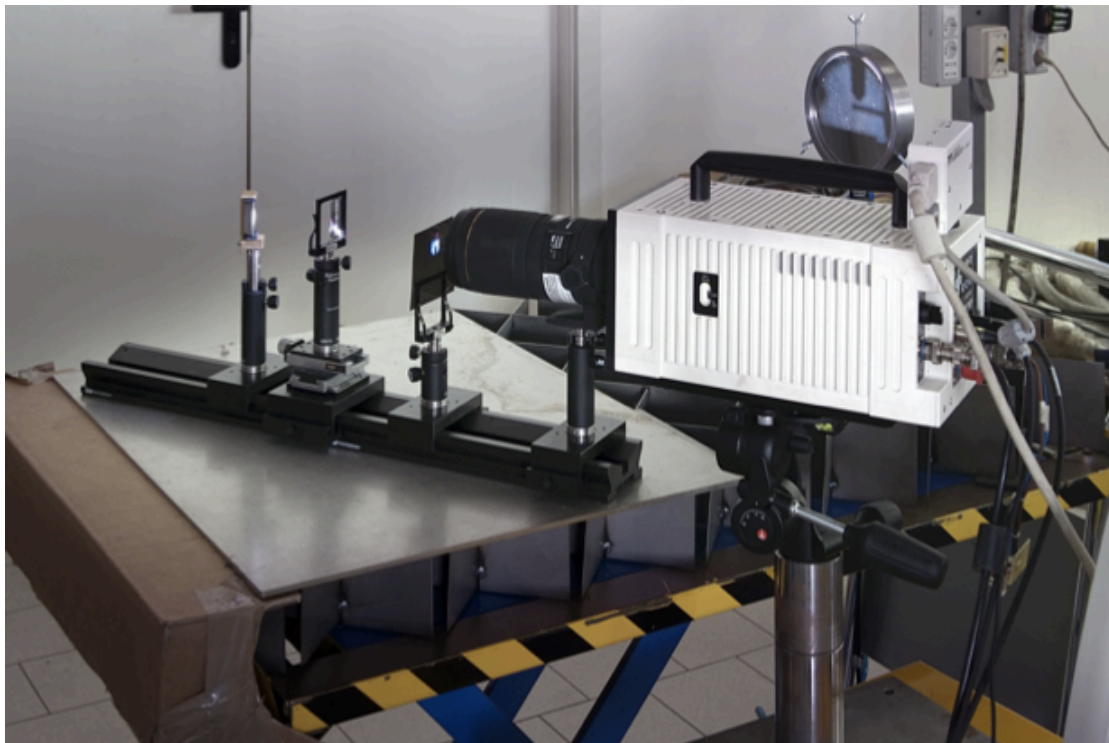
Fig. 4: Picture of the experimental Schlieren setup. At increasing distances from the lens of the camera: a neutral density filter, the knife and one of two small secondary mirrors. It can be seen also in the second floor of the second parabolic mirror, on which it is visible the shadow of the torch and of the workpiece.
