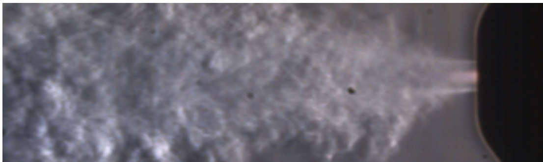
Fig. 6 – Schlieren images of the flow at the cutting torch nozzle outlet during pilot arc phase – Acquisition at 5000 fps. Horizontal knife-edge.
