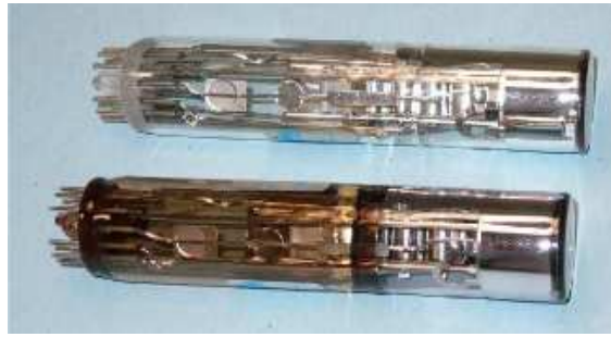
Figure 3.12: Two PMTs. The one in the upper part is a not-irradiated reference PMT. The one in the bottom part has been irradiated with gamma dose. The most striking change is the visible darkening of the glass part of the PMT. The quartz part kept its initial transparency.
