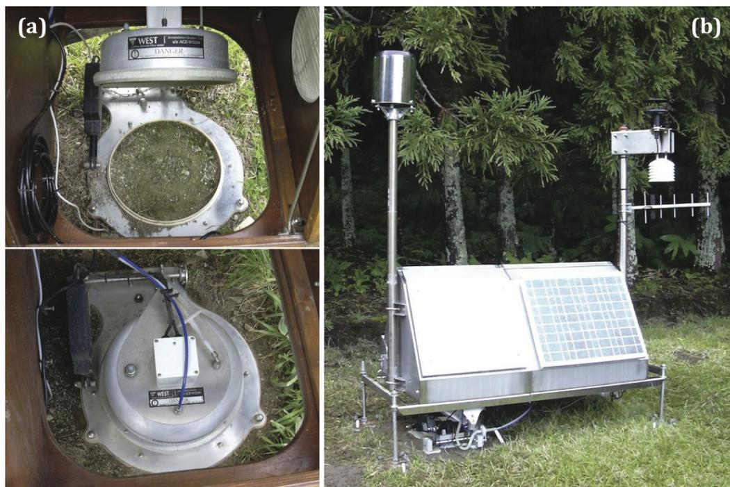
**Figure 6.2:** (a) Monitoring site showing the accumulation chamber in up and down positions; (b) Shelter of GFUR2 with the solar panel. Several meteorological sensors are coupled to the station.
