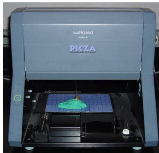
Fig. 2. Roland PICZA PIX-30 piezoelectric digitizer. From the Laboratory of Anthropology at the University of Arkansas (USA).
