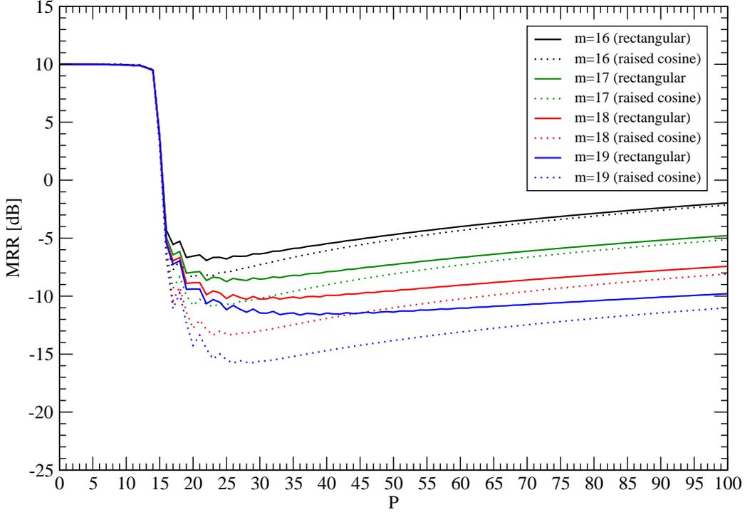
Fig. 2.2: Pseudonoise method. MRR as a function of the number of taps  $P$  when the coupling channel has only one tap: comparison between rectangular and raised cosine filtering for different values of the length of sequences  $M$ .
