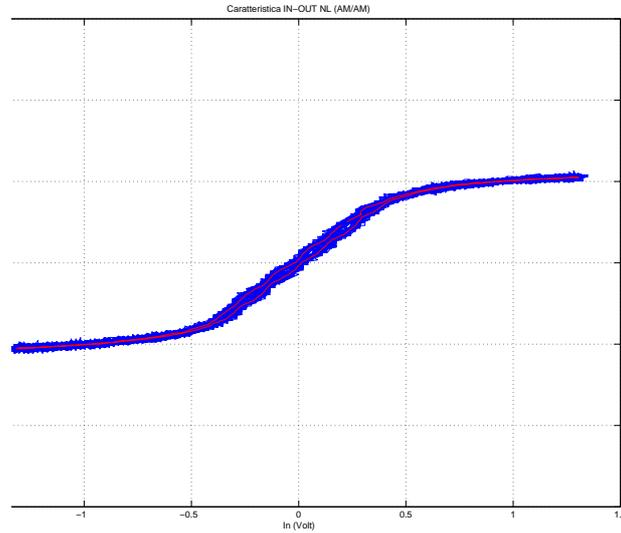
Fig. 3.6: Input-output characteristic of the non-linear element.  $I_{BO} = 15\text{dB}$ .  $\gamma = 0.001$ .
