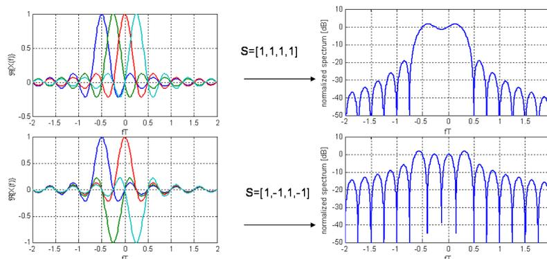
Fig. 3.1: OOB radiation as depending on the symbol sequence  $S$ . A very simple example ( $N = 4$ , BPSK modulation): on the left the contributions of each symbols in the frequency domain are depicted and on the right the related spectrum is shown. It is evident as the OOB of the sequence with alternate sign is much more higher with respect the sequence with the same sign
