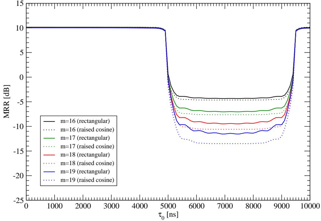
Fig. 2.4: Pseudonoise method. MRR as a function of the coupling channel delay  $\tau_0$  (only one tap channel is supposed): comparison between rectangular and raised cosine filtering for different values of the length of sequences  $M$ .
