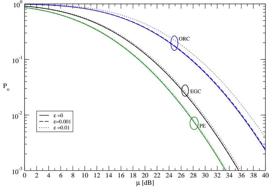
Fig. 1.9: BEO vs  $\mu_{\text{dB}}$ , for different estimation errors  $\varepsilon \triangleq \sigma_{\text{E}}^2/\sigma_{\text{H}}^2$  and  $P_{\text{b}}^* = 10^{-2}$ . Comparison among different combining techniques.
