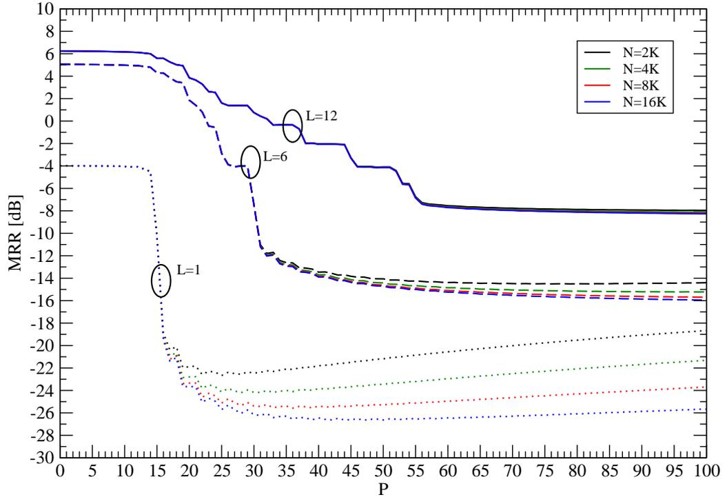
Fig. 2.7: Pulse method. MRR as a function of the number of taps  $P$  when the coupling channel is modeled as TU12 and 1,6 and 12 echoes on 12 are considered respectively: comparison between different values of the number of accumulations  $N$ .
