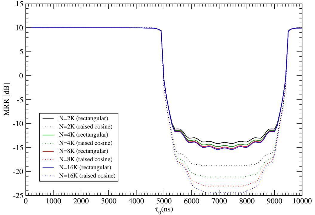
Fig. 2.5: Pulse method. MRR as a function of the coupling channel delay  $\tau_0$  (only one tap channel is supposed): comparison between rectangular and raised cosine filtering for different values of the number of accumulations  $N$ .
