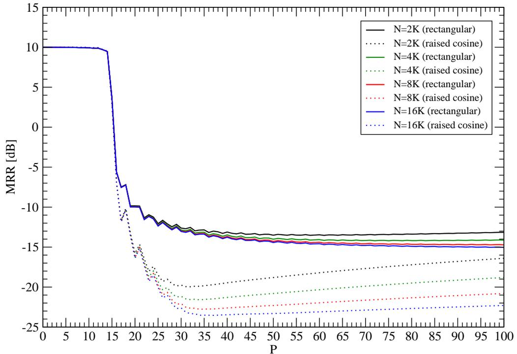
Fig. 2.3: Pulse method. MRR as a function of the number of taps P when the coupling channel has only one tap: comparison between rectangular and raised cosine filtering for different values of the number of accumulations  $N$ .
