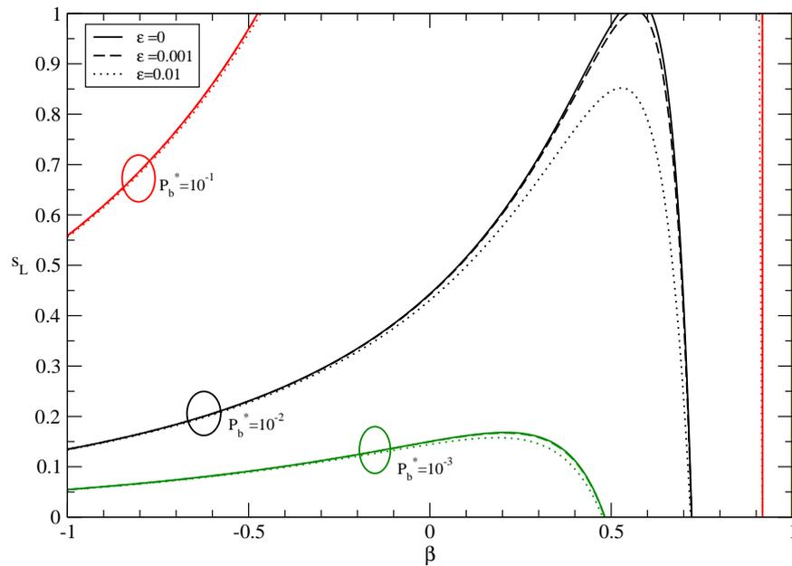
Fig. 1.7: System load vs.  $\beta$  giving the target BEP  $P_b^* = 10^{-1}$  (red),  $P_b^* = 10^{-2}$  (black), and  $P_b^* = 10^{-3}$  (green), for different normalized estimation errors  $\varepsilon \triangleq \sigma_E^2/\sigma_H^2$ .
