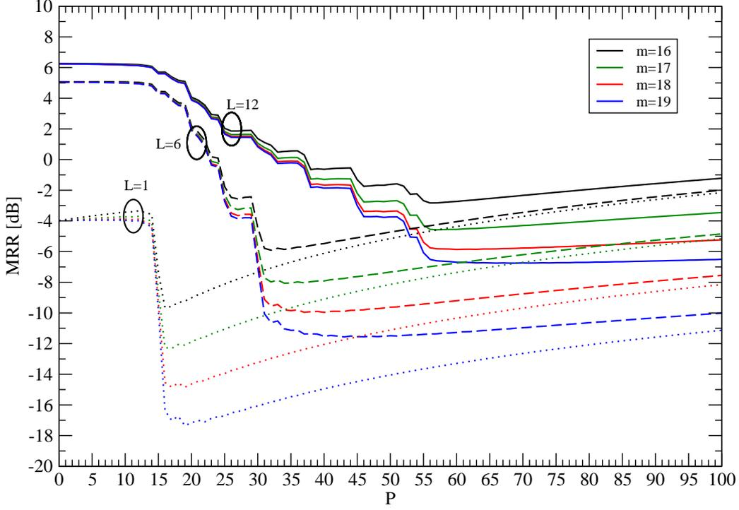
Fig. 2.6: Pseudonoise method. MRR as a function of the number of taps  $P$  when the coupling channel is modeled as TU12 and 1,6 and 12 echoes on 12 are considered respectively: comparison between different values of the length of sequences  $M$ .
