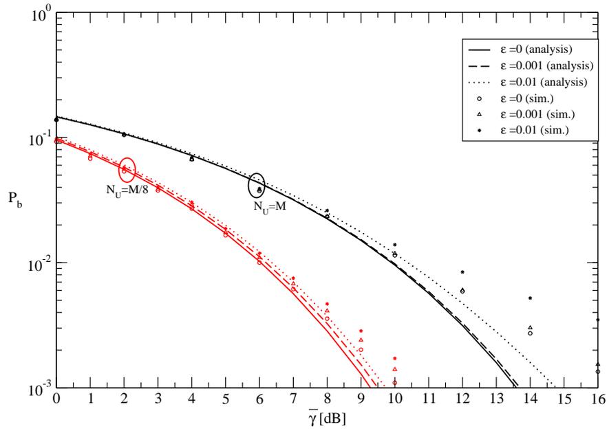
Fig. 1.5: BEP vs. the mean SNR  $\bar{\gamma}$  adopting the optimum  $\beta$  in case of perfect CSI, varying the normalized estimation errors  $\epsilon \triangleq \sigma_E^2/\sigma_H^2$ : comparison between  $N_U = M = 1024$  and  $N_U = M/8 = 128$ , with  $L = M/16$ .
