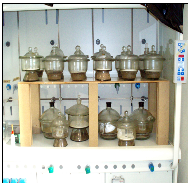
Figure 3.1.4.4. Desiccators used for the biodegradation of imidazolium-based ionic liquids in soils.
