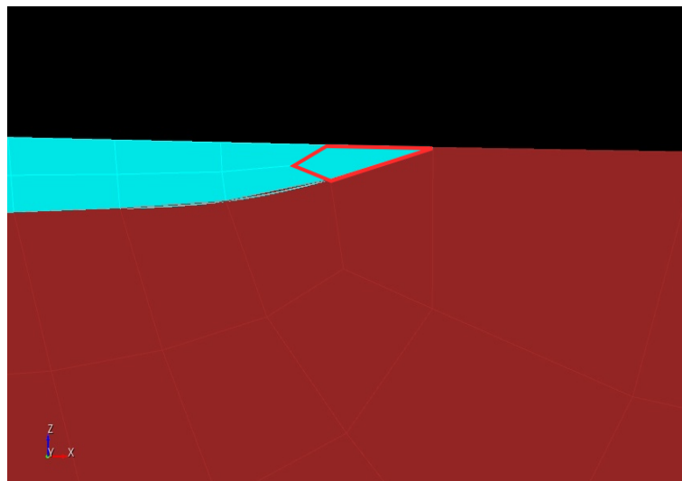
Figure 4.7: In this picture we possible to see the problems related to the zones of connection between bedrock and earth surface models: elements used to mesh the ice layer have linear dimension of 50m , nevertheless at least one element - in figure the one with red edges - with a bad equiangle skewness is created.
