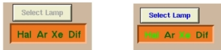
Figure 12 - All lamps OFF and the diffusor in Close position (left) Halogen and Xeno lamps ON (right).
