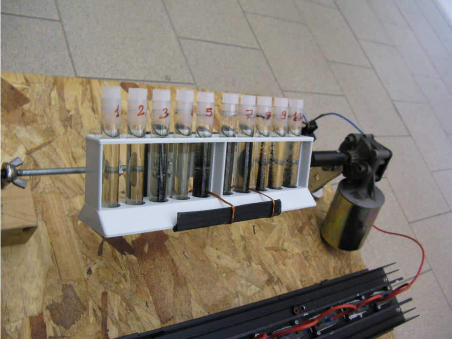
Figure C.7: Homemade mixer used to guarantee initial uniform concentration in the test-tubes.
