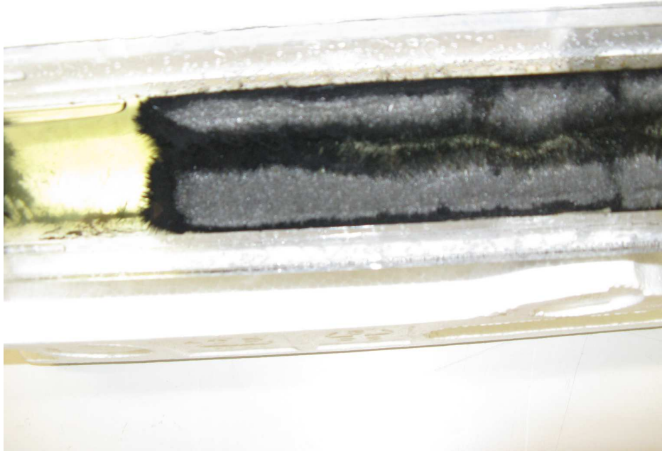
Figure 3.5: Picture of a filter packaged in the wrong way: a channel through with the flow is facilitated is visible.
