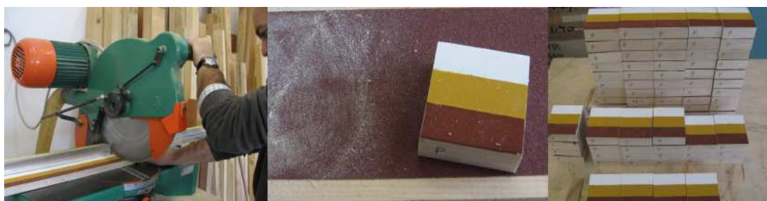
Fig.3.16. Cutting the boards and polishing with sand paper
