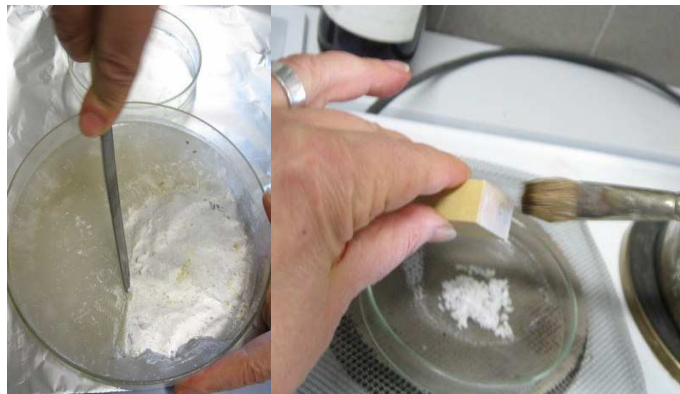
Fig.3.23. Preparation for paraffin wax and put paraffin wax by brushing
