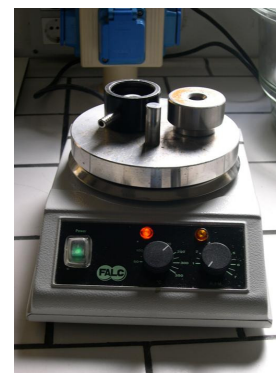
Figure 4.7: The heating of the Anvil Die on a hotplate of a magnetic stirrer.
