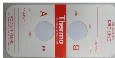
Figure 4.13: Picture of the PE thin film from Thermo Electron Corporation with two circular areas (21 mm diameter) for sample application.
