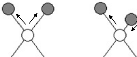
Figure 2.4: Symmetric and asymmetric stretching vibration of a molecule are changes along the interatomic bond axis [23].
