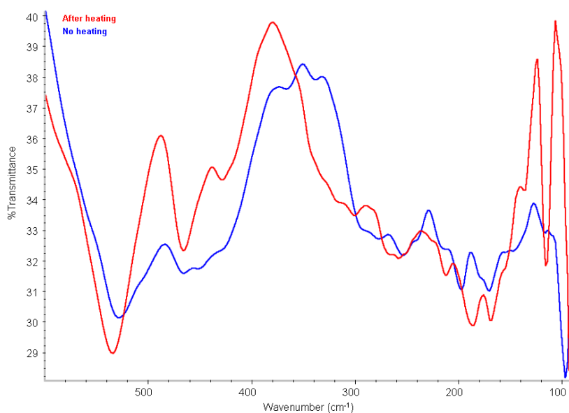
Figure 4.28: Spectra of Iron blue Vivianit ( \text{Fe}_3(\text{PO}_4)_2 \cdot 8\text{H}_2\text{O} ) without (red) and after (blue) heating. The chemical structure of vivianit has clearly changed.
