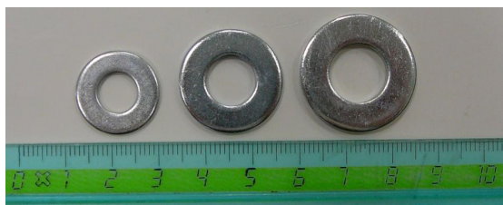
Figure 4.9: Various sizes of O-rings employed as sample forms with inner diameter of 8, 10 and 13 mm and 1 mm thickness purchased from a everyday ironmonger shop.
