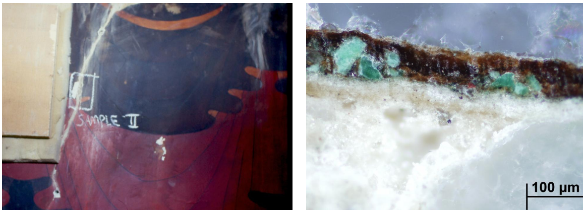
Figure 7.13: Photo of sampling area of T2 on blue drapery and microscopic photo of cross-section of sample T2 (original magnification 200x) showing dark blue/brown layer with inclusions of green crystals.
