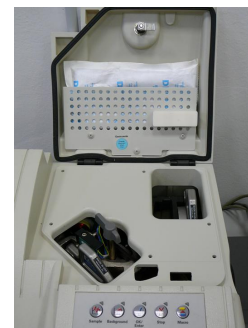
Figure 3.6: The beamsplitter compartment with easily exchangeable beamsplitter for MIR and FIR region.
