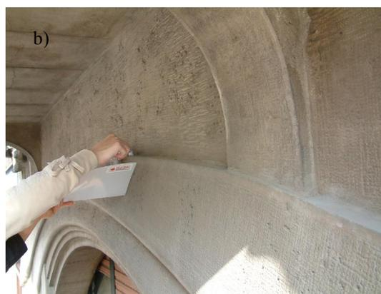
**Figure 3.11.** Casa Galleria Vichi. Sampling point, (a) and (b) incoherent grey deposit, easily collected by brush
