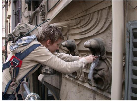
**Figure 3.9.** Sampling: (a) platform lift, (b) collection of the black crust from area protected from rain ran-off.
