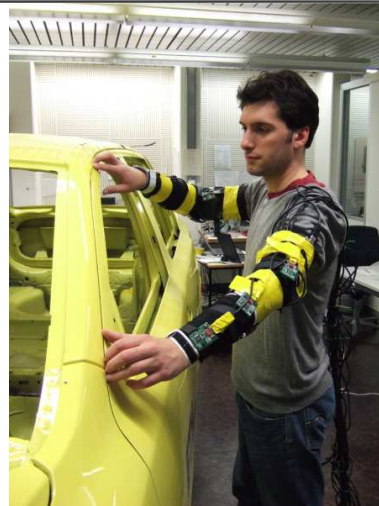
The user checks the gaps on the front door by sliding his left and right hand over the gaps. The two hands move simultaneously.
