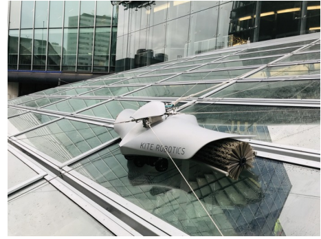
(d) Kite Facade Inspection System (Source: Kite Robotics).
