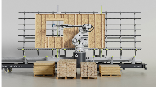
(b) MicroFactory for on-site home assembly (Source: AUAR).
