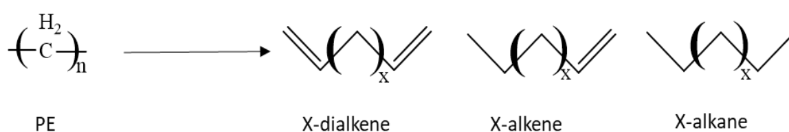
Scheme 4.1. Main thermal degradation products of PE.
