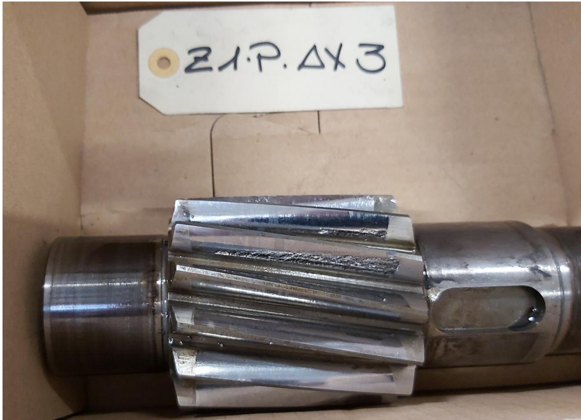
Figure 67 - Detail showing pitting on the AX3 pinion, last stage, Test7B.
