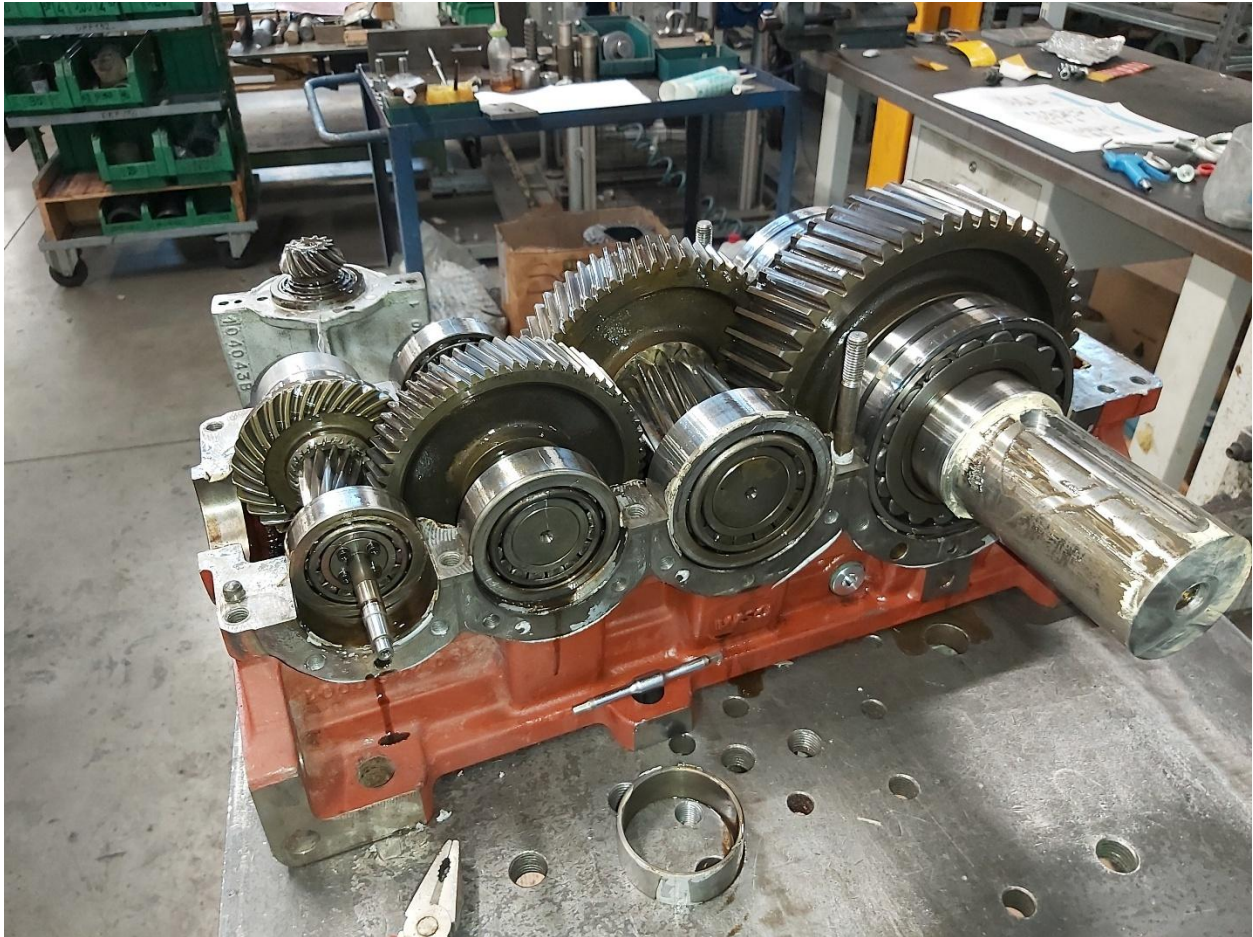
Figure 65 - Photo of the gearbox after disassembly at the end of the test, Test7B.
