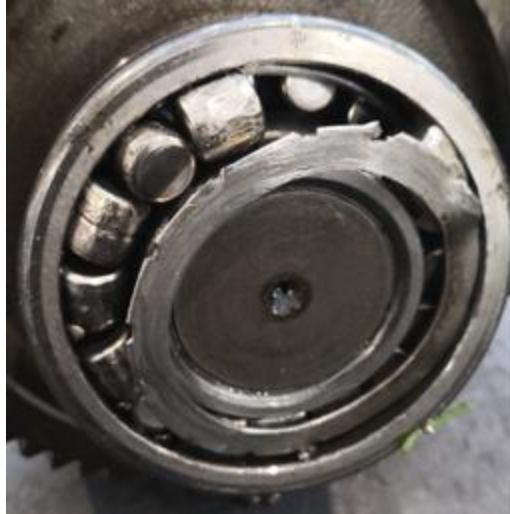
Figure 74 - AX3 bearing after the first teardown at 3135.5 Working Hours
