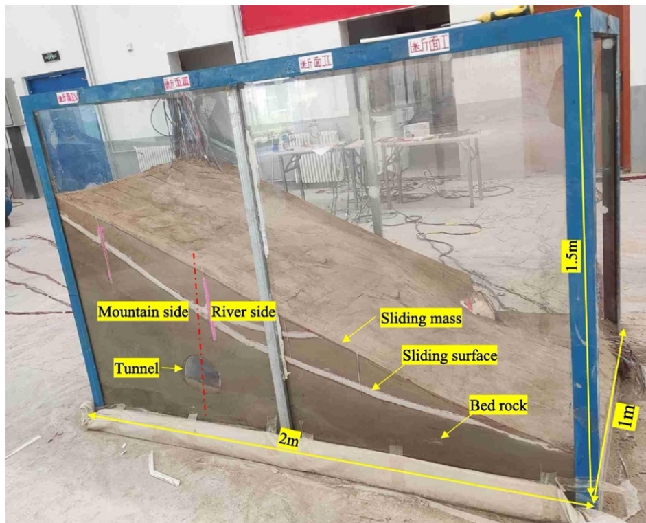
Figure 8 - Complete physical model of a tunnel involved in a landslide (Wei et al. 2023)
