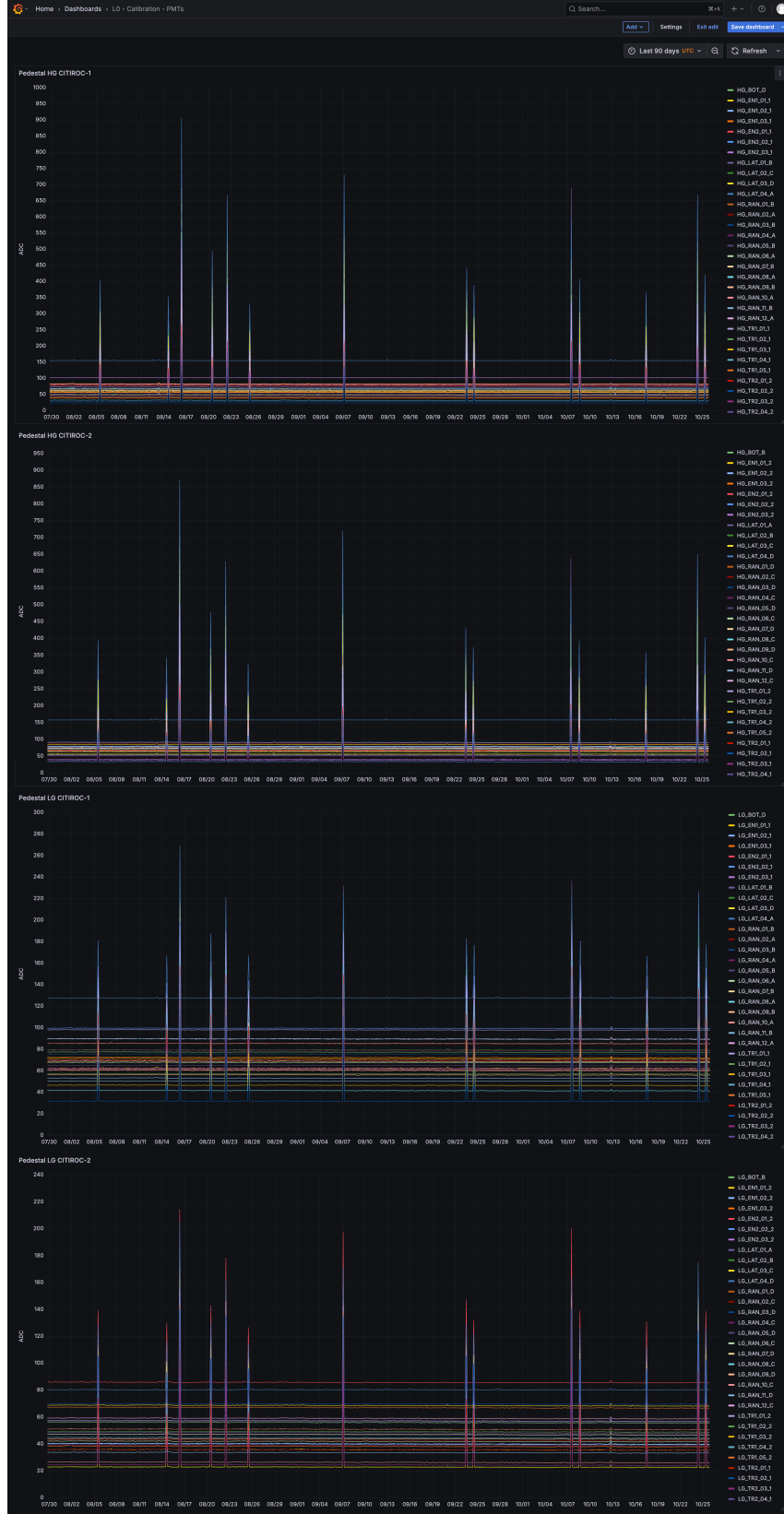
Figure 5.2.2: Example plots of PMTs’ pedestals measured during calibration. On top 2 panels: the pedestals measured in the HG scale for PMTs read-out by CITIROC-1 and CITIROC-2, and on bottom 2 panels are the pedestals measured in the LG scale for PMTs read-out CITIROC-1 and CITIROC-2.
