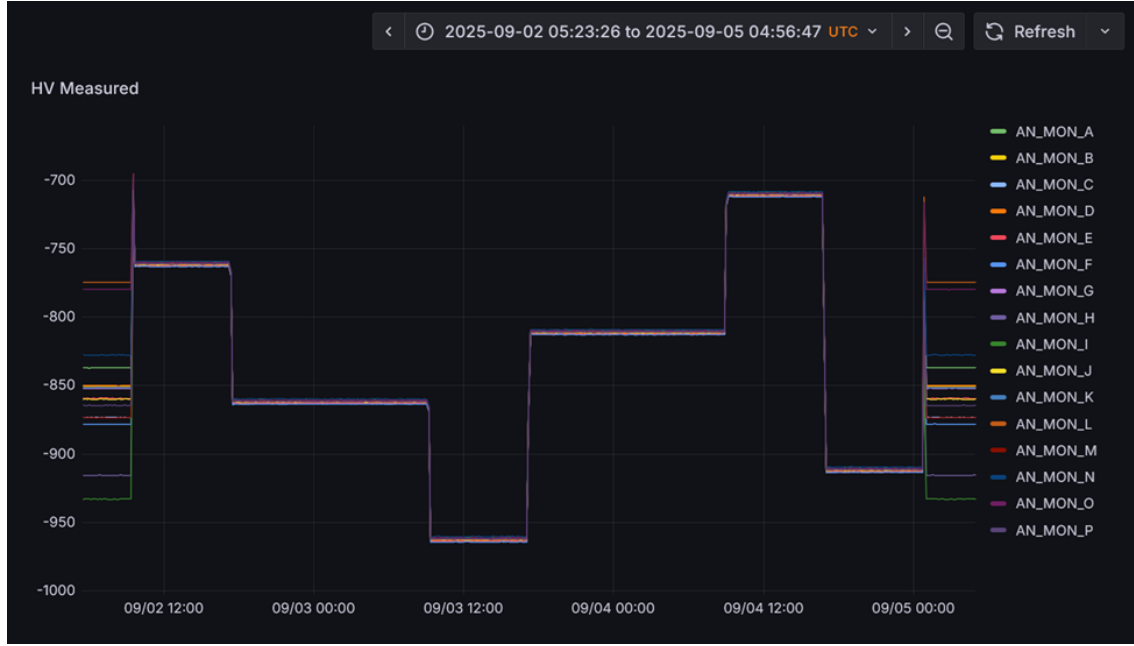
Figure 5.3.1: The HV monitor showing the scanning procedure featuring the 6 stages with equal HV for all the PMT lines.
