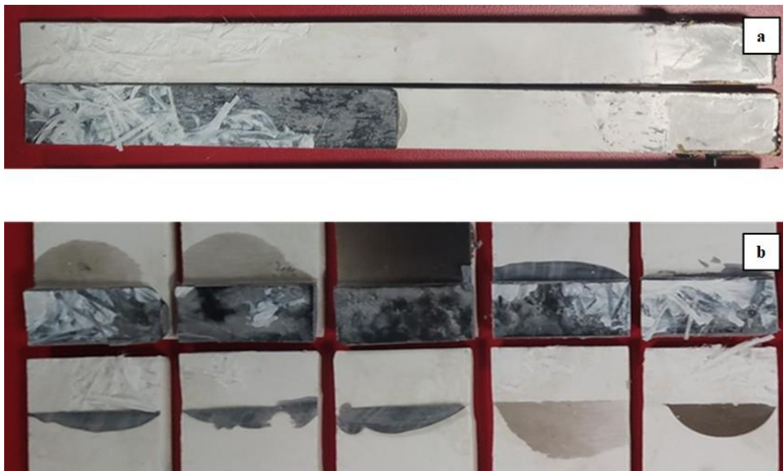
Figure 39: Fracture surfaces from different adherend material analysis: a) DCB specimens and b) SLJ specimens
