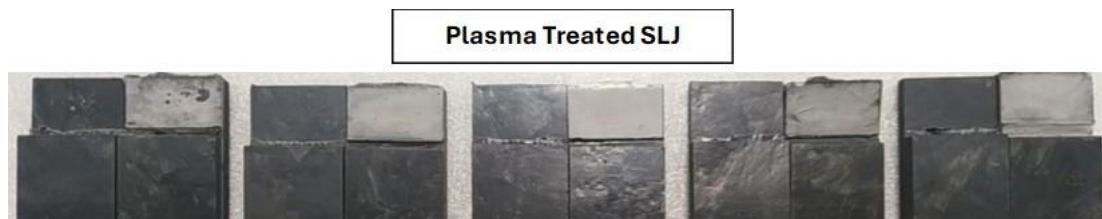
Figure 26: Fracture surfaces of plasma treated SLJ specimens: a difference in colors may be observed on SMC bare adherend, debonded surface with thin-veil adhesive and adhesive layer. Also, on the first specimen from the left, small patches of detached adhesive material are visible.
