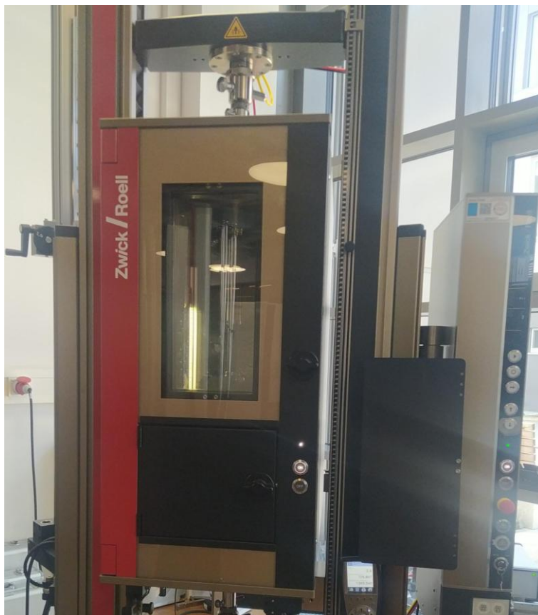
Figure 32: Temperature chamber employed for DCB and SLJ in temperature tests (-10 and +85 °C)
