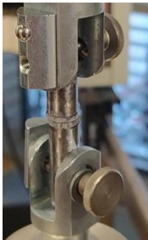
Figure 56: Testing of Rod Joint specimen
