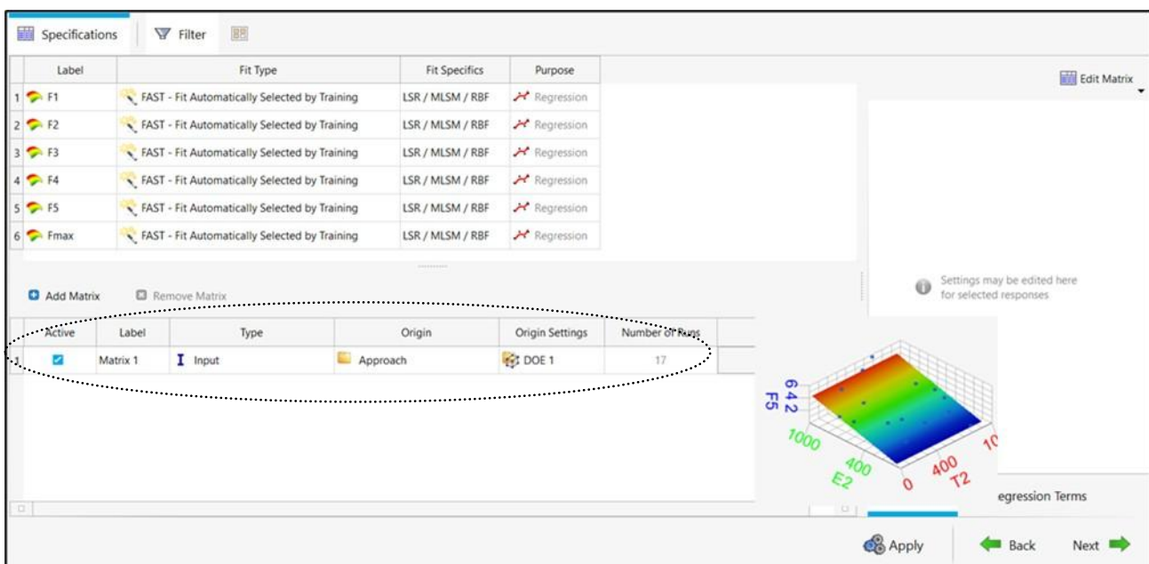
Figure 71: List of possible FIT algorithms, with particular focus on the selection of the inclusion matrix, necessary to read and process data without simulation and to generate an optimal "Response Surface"
