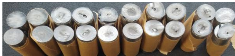
Figure 63: Rod Joint specimen after fracture at peak load
