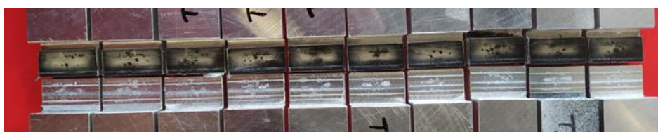
Figure 62: Thick Lap Shear specimen after fracture at peak load
