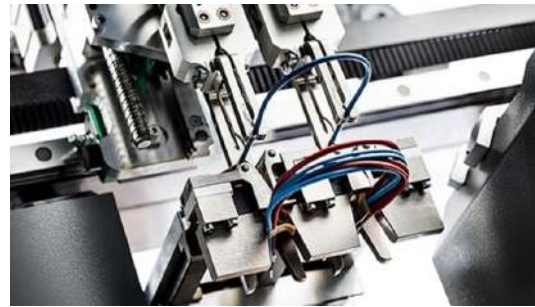
(b) End-line KomaxZ640, its gripper with the final cable product.
