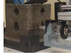
(d) Second iteration failed due to wall contact.
