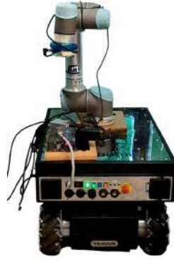
Figure 4.11. Simulation model of the mobile manipulator, consisting of an omnidirectional base and a 6-DOF UR robotic arm.
