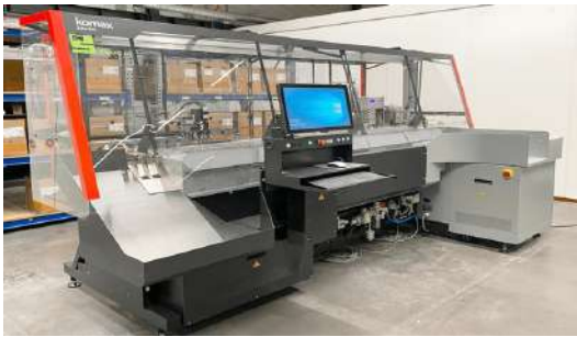
(a) Komax ZETA 640 cable production machine.
