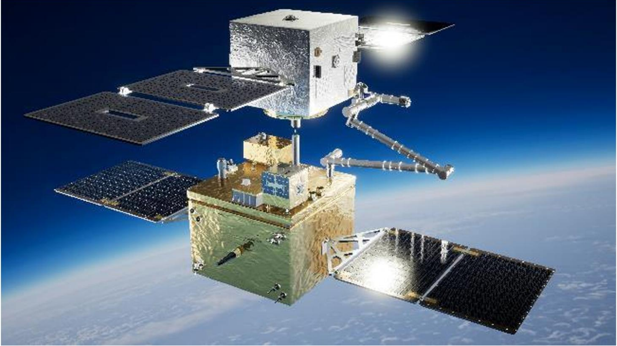
Figure 3.1: Artistic rendering of the EROSS spacecraft during close-range proximity operations, illustrating the robotic servicing arm and modular spacecraft components in orbit [20].
