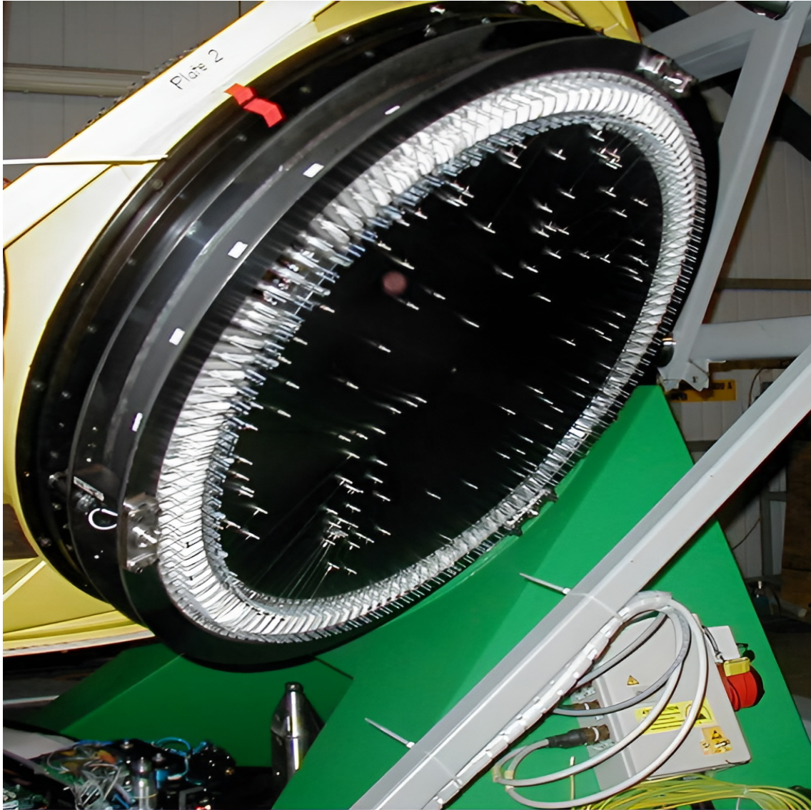
FIGURE 2.10: Picture of FLAMES in GIRAFFE MEDUSA mode. View of the back of one OzPoz plate where all the fibers are attached with magnetic buttons. Credits: ESO.
