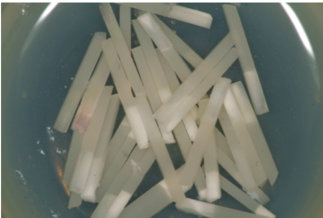
Fig. 3. The sticks are collected and, in the case of artificial aging, divided into baseline and aged groups. Each stick consists of one part dentin and one part resin composite, separated by the adhesive interface, which is subjected to tensile stress during testing.
