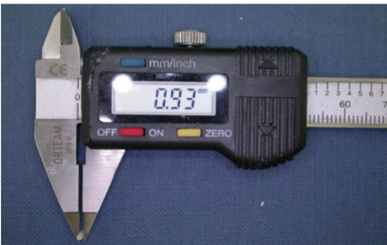
Fig. 5. Measurement of the stick dimensions using a digital caliper.
