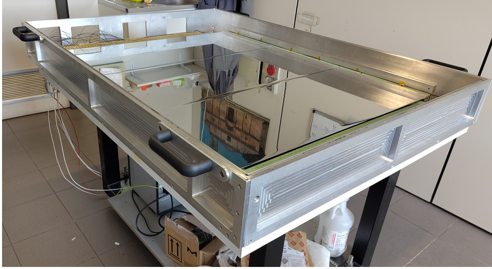
Figure 4.25: View of the lateral walls of the gas box.
