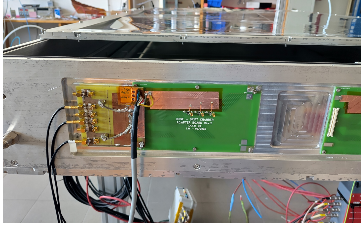
Figure 5.5: The 12-channel board mounting two VTX preamplifiers during the tests in Ferrara.
