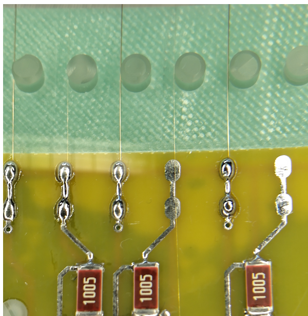
Figure 4.21: Detail of the pads of a PCB board: four of them have the wire already welded, while the fourth from the left has the anode wire stretched across it. All the wires are touching the plastic pins.
