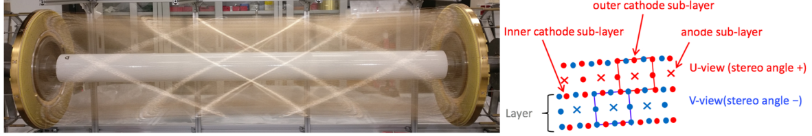
Figure B.6: Left : the entire drift chamber with all layers mounted. The hyperbolic profile of the chamber is visible. Right : drift cells configuration.
