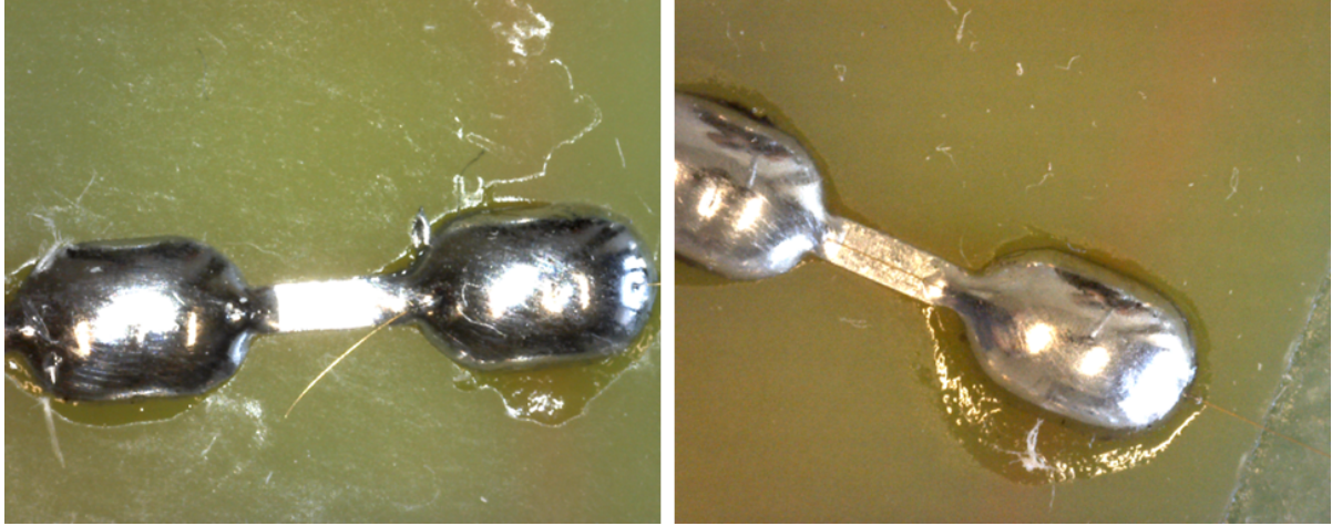
Figure 4.28: Left : a sense wire broken between the two welds. Right : the sense wire is properly soldered, a small white lint is visible below the rightmost weld.
