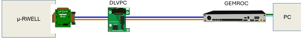
Figure C.22: Scheme of the connections of the TIGER-GEMROC system. The Low Voltage cable is indicated in red, the data cable in blue. Between the FEB and the FPGA there is the DLVPC card.
