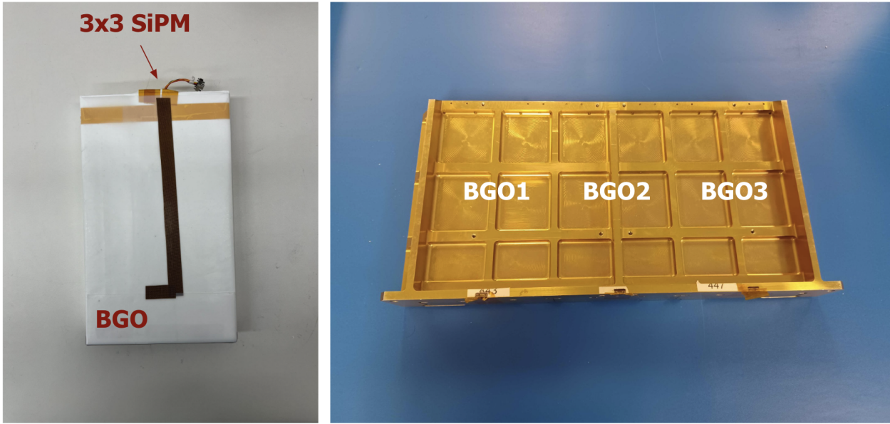
Figure 5.1 – Wrapped BGO crystal with coupled SiPM array on the left (picture taken at NRL) and the EM X-wall with the three BGO crystals on the right (picture taken at SSL).
