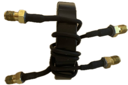
(b) Lateral view of the implemented transformer.
