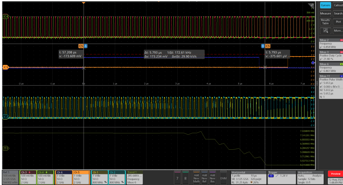
Figure 4.47: Measured ISR-to-actuation delay under a stepped update condition.
