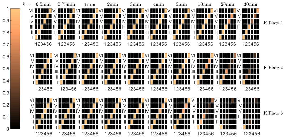
Fig. 5.12 MAC plots for kantele plates (K.Plates) compared against the baseline configuration. Each column corresponds to a different plate thickness, while each row represents an increasing surface area: Plate 1 ( A = 1.39 \text{ m}^2 ): red line with plus markers; Plate 2 ( A = 0.34 \text{ m}^2 ): blue line with diamond markers; Plate 3 ( A = 0.08 \text{ m}^2 ): green line with dot markers, from top row to bottom.
