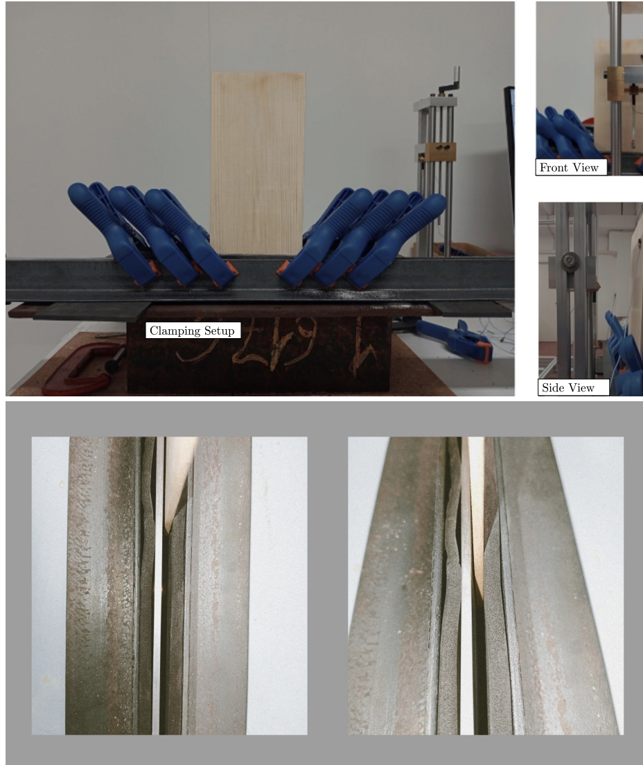
Fig. 3.4 Experimental setup for the tonewood sample with BCs = \{C-F-F-F\} and \alpha = 223/114 , whose modal coefficients are provided in Table 3.2. The impact hammer is mounted on a pendulum that halts after recoil to prevent multiple impacts. The protective rubber pad used in the clamping system is visible below.
