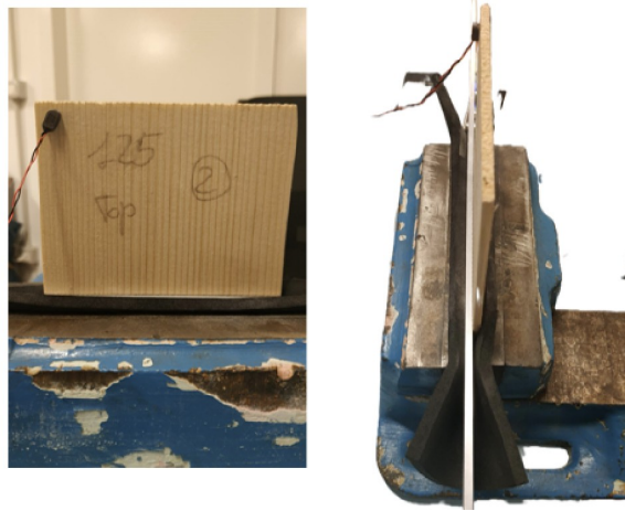
Fig. 4.11 Tonewood sample used in guitar making, here set under cantilever BCs.
