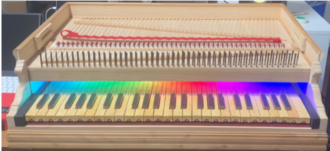
Figure 2.16: Mark I demonstrating the addressable RGB LED array.
