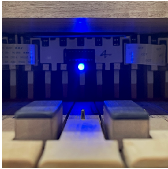
Figure 2.22: RGB LEDs behaviour in calibration mode. LEDs are aligned with the keys and colour-coded for quick identification of the jack being calibrated and its state.
