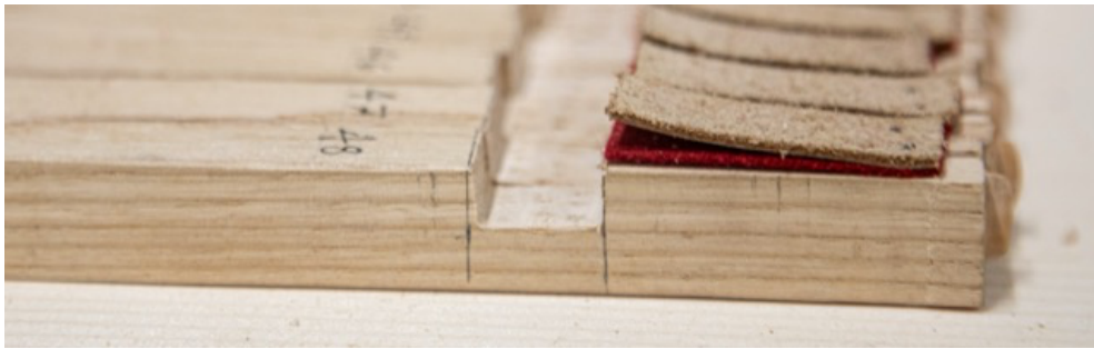
Figure 2.21: Mark I keys after milling and re-finishing.
