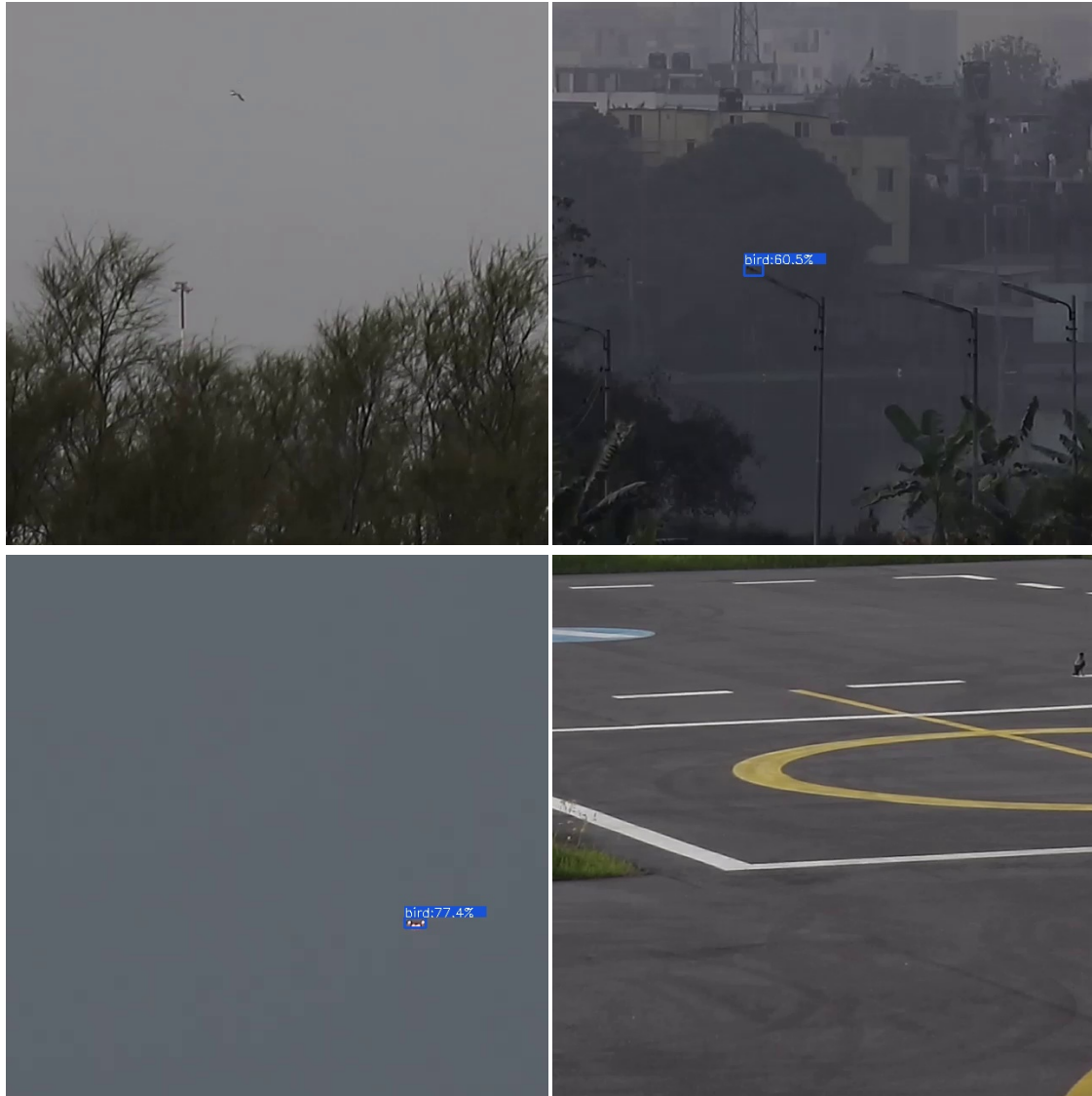
Figure 5.6: Failure cases. Highlights of typical failure cases, including missed birds and false positives. The model occasionally confuses birds with similar-looking objects (a drone and a street lamp head) or fails to detect birds in flight or on the ground.
