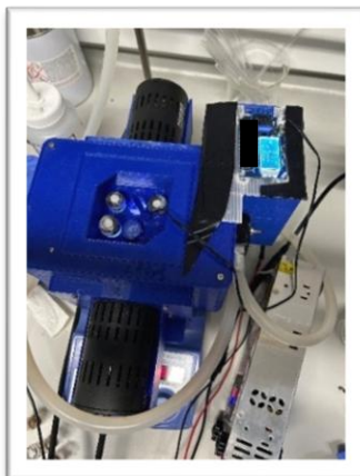
Figure 3.31. Reaction setup using 3D-printed photoreactor 81 with 390 nm Kessil lamp.
