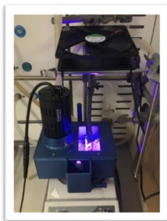
Figure 2.33. Kessil lamp set-up for the quantum yield determination
