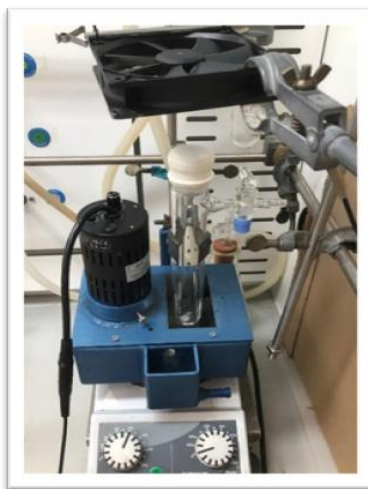
Figure 2.25. Setup for the gram-scale experiment using PhotoRedOx Box TC™ reactor with 390 nm Kessil lamp
