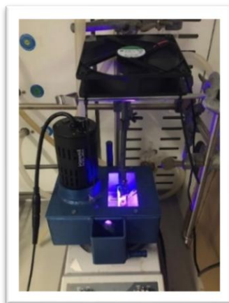
Figure 3.35. Kessil lamp set-up for the quantum yield determination
