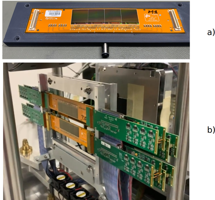
Figure 3.9: a) A module of 4 M28 chips with electronics, which forms one of the two extensions of a ladder. b) View of the two planes of the IT in the CNAO 2023 configuration, followed by VT.
