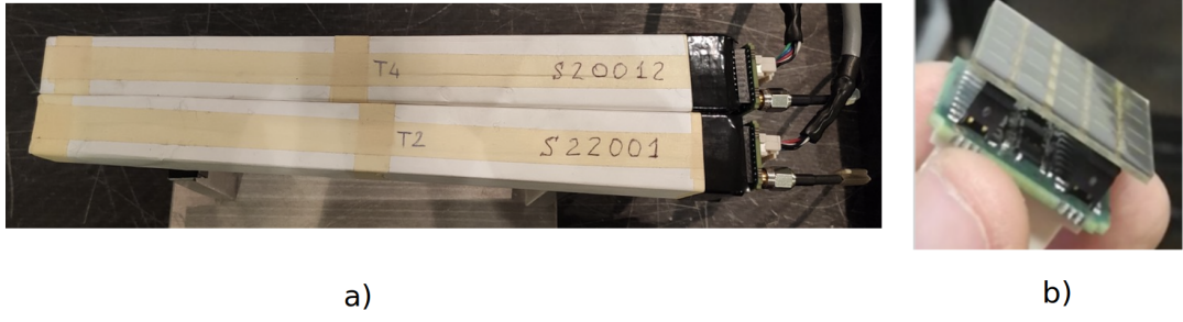
Figure 3.12: a) Module of two BGO crystals, coupled at one end to SiPM and its readout. b) Picture of the SiPM used for energy measurements.
