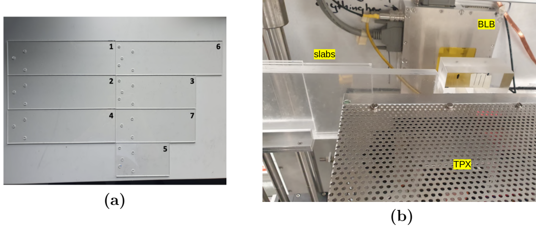
Figure A.10: a) PMMA slabs for WET calibration. b) Combination of the slabs to be put after the BLB and before the TPX sensors for an open field imaging. From [154].
