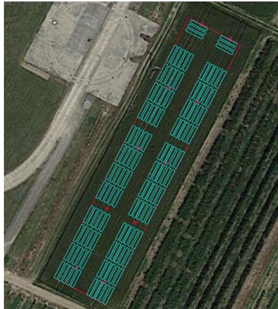
Figure 4. Final representation of the imported CAD layer into QGIS ensures centimetre-accurate sowing and provides a spatial framework for integrating future drone imagery and soil-property maps.
