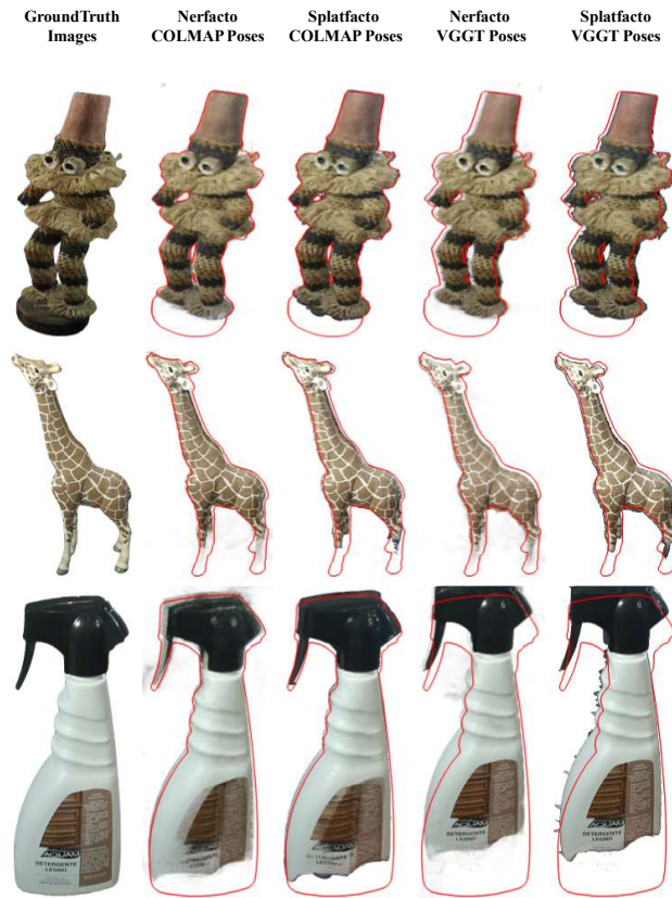
Figure 6.5: Qualitative NVS results. Red edges denote the ground-truth object masks. Renders based on VGGT poses show visible misalignment with the mask due to pose inaccuracies, whereas COLMAP poses produce better alignment and higher-quality novel views.
