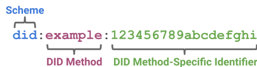
Figure 2.3: A simple example of a decentralized identifier (DID)
