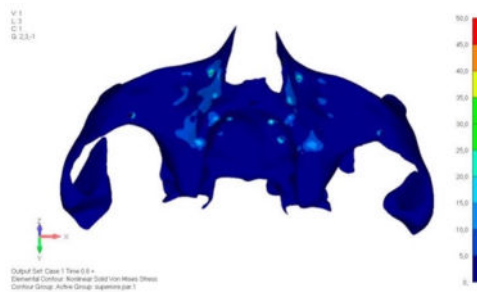
Figure 10. Upper jaw model V0 subjected to load configuration 2, representing a low-stress scenario with force applied exclusively to the posterior dentition.
