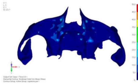
Figure 9. Upper jaw model V0 under load configuration 1, representing the least critical scenario with force evenly distributed across the full dental arch.
