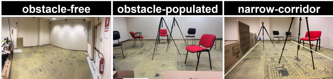
Figure 4.7. Environments for in-field testing. The test arena is 6.6 \times 5.6 \text{ m}^2 wide, restricted to 1.95 \times 4.5 \text{ m}^2 for the narrow-corridor scenario.
