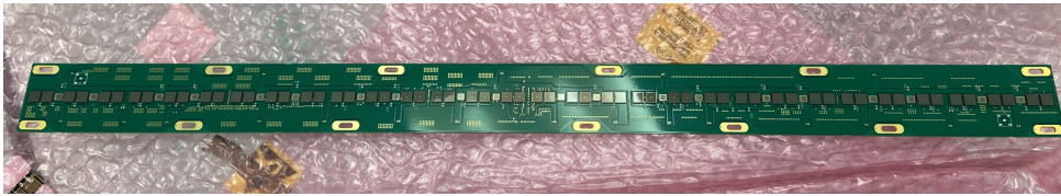
Figure 2.10: PCB hosting the SiPMs to read out a US plane side.
