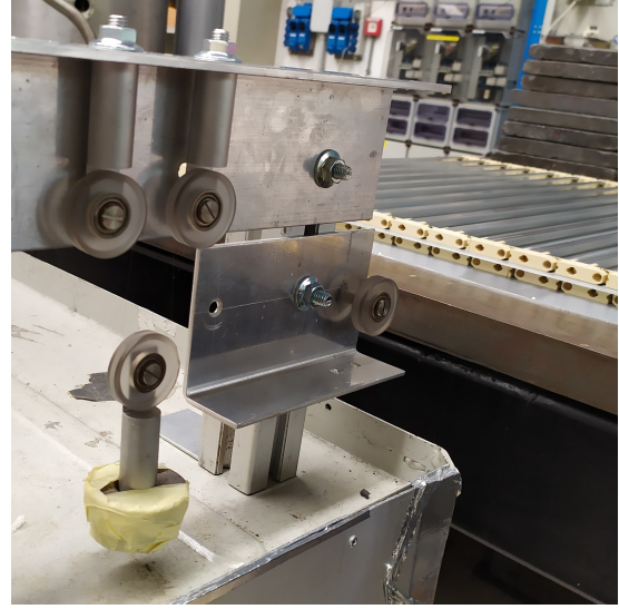
Figure 6.4: Tool used to tension the wires during the MiniDTs' assembly.
