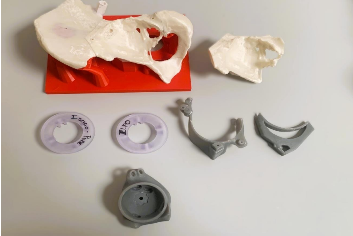
Figure 5: 3D printed phantom and Patient-specific Instruments (PSIs)
