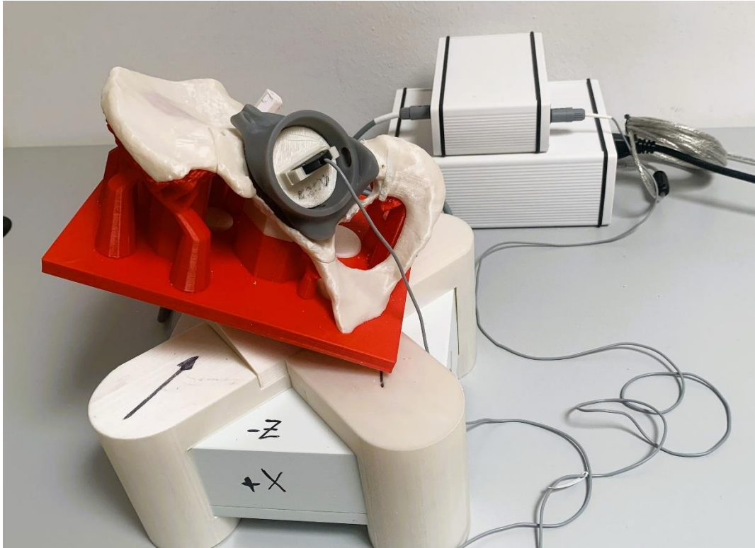
Figure 6: NDI Aurora Tracking System for post-implantation measurement of inclination, anteversion and displacement along x,y and z axis.
