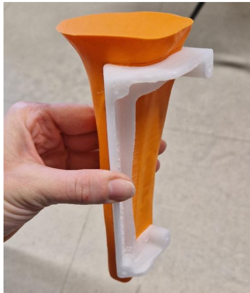
Figure 37. Non-sterile 3D printed guide (white) tested on the bone model (orange).
