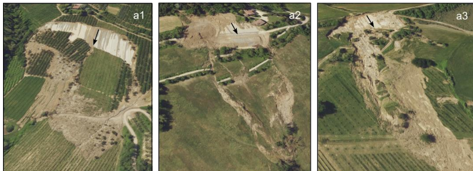
Figure 3.5. Representative images of the two distinct types of debris slides caused by the May 2023 event.
