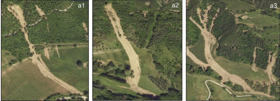
DF2) Debris flows with runout limited on steep forested slopes
