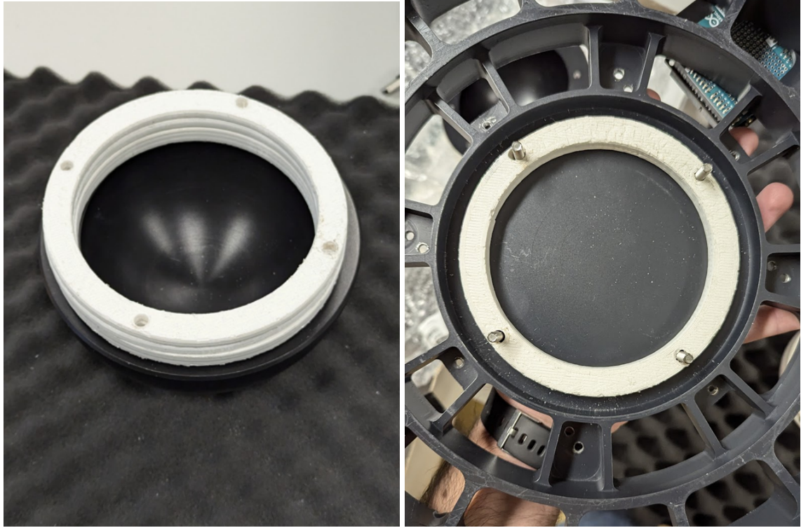
Figure 3.14: Spacers used to shift up the CM position. The picture on the left shows the spacers on the air bearing module, the picture on the right shows the spacers on the 1U platform
