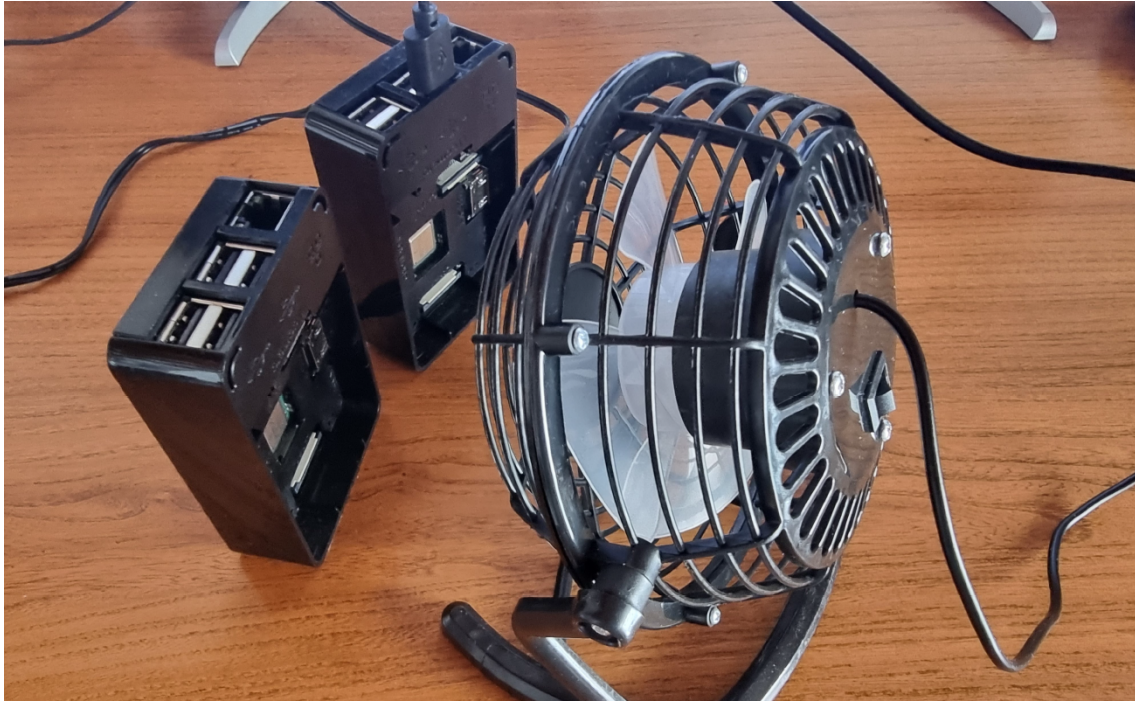
FIGURE 4.2: Cooling mechanism for Raspberry Pi devices.
