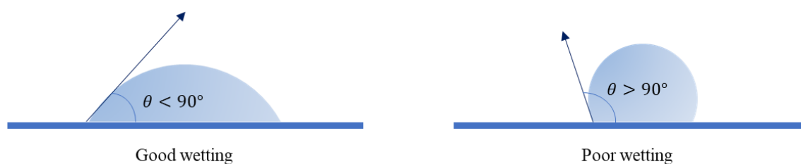
Figure 3.6. Wetting behaviour of different solid/liquid interfaces and associated contact angle values.
