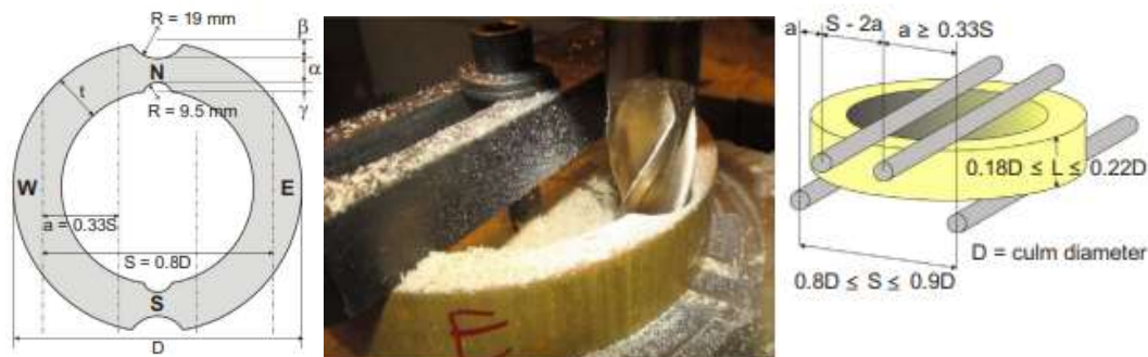
Figure 50 Flat ring flexure specimen (a and b) and test (c) in the reference experimental study [121]
