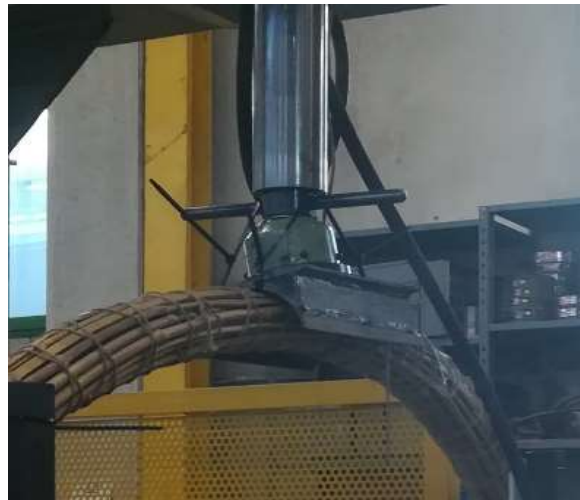
Figure 107 Lateral thrust of the loading cell which causes the interruption of the test
