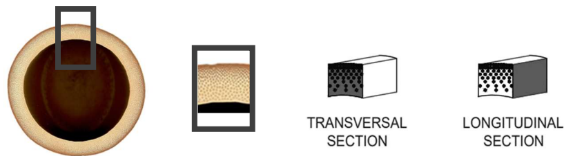
Figure 27 Provenience of the sample into the section of the culm
