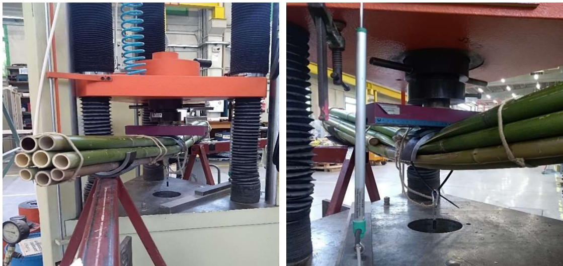
Figure 92 Details of the set-up and the beam during the execution of the test. On the left, the instrumentation to measure the displacement and the transmission of the load is shown. On the right, detail of the support of the beam,
