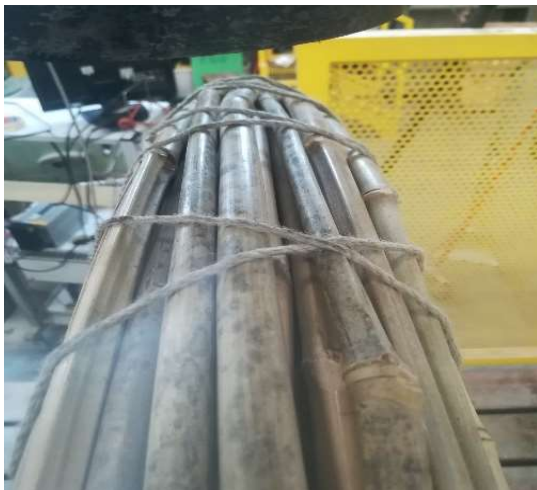
Figure 106 keystone point after the execution of the test. No visible signs of damage are visible
