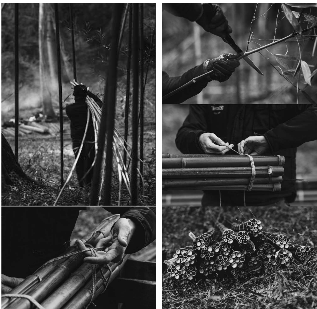
Figure 83 Harvesting of the canes and creation of the modulus. Images courtesy of Arundo Costruzioni Organiche
