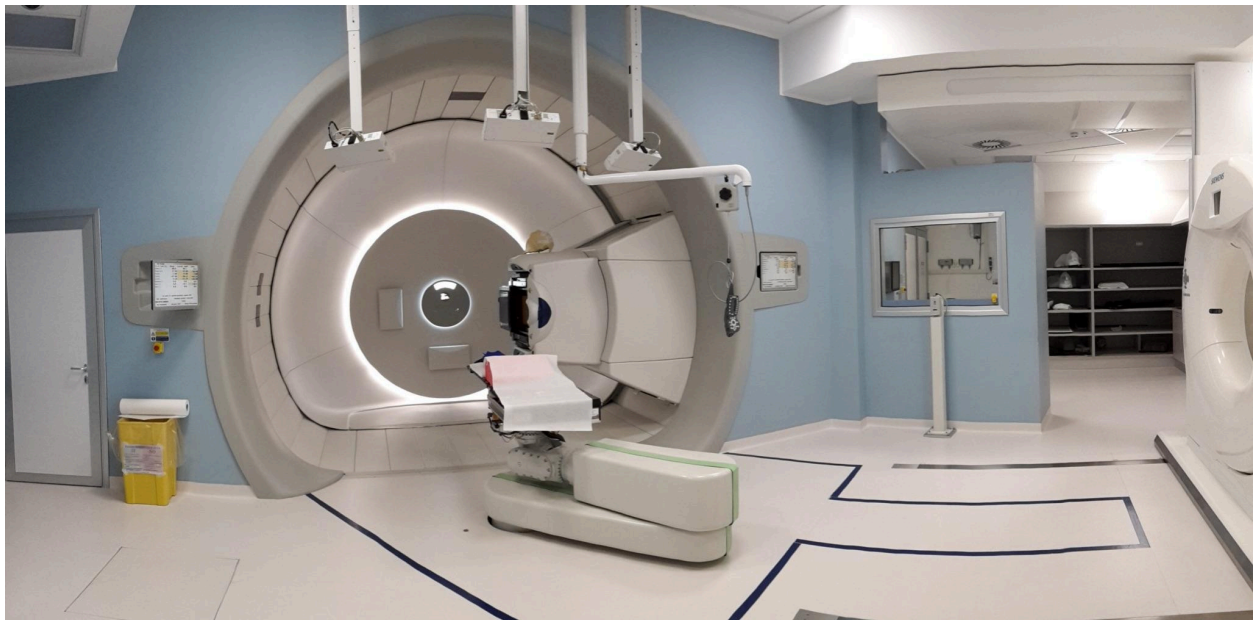
Figure 2: The CT-on rail (right side) of the Trento facility in gantry room 1.
