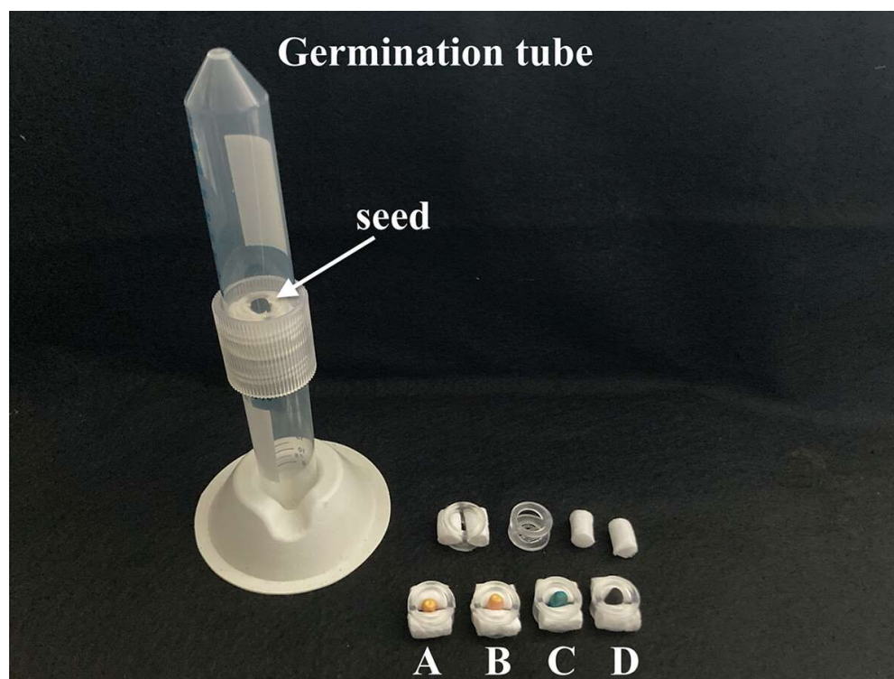
Figure 3.5.3 Corn seed germination and seed water uptake studies were carried out using a specifically designed test tube system (left). Seeds (A: control; B: dewaxed; C: commercially treated; D: biochar treated) were secured between two cotton plugs at the junction of two test tubes held together by a threaded sleeve created with a 3D printer.
