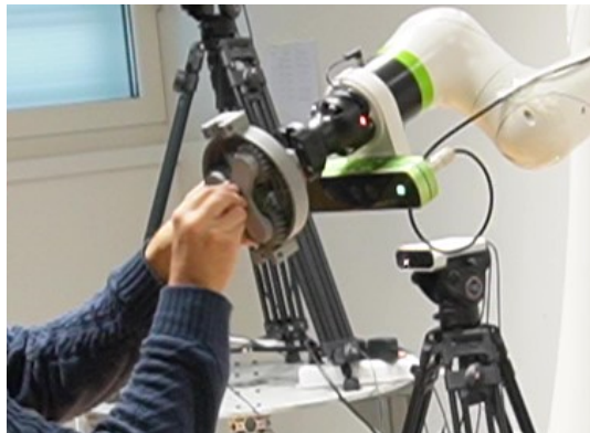
FIGURE 4.6: A detail of the joint action where the user focuses on the correct meshing of the gears while the cobot helps keeping the parts in place as a third hand.
