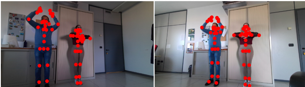
FIGURE 3.5: Two RGB-D cameras capture the User from two different points of view and the Interpreter uses the depth video to extract the skeletal joints position, useful to infer an index of physical energy consumption and fatigue.
