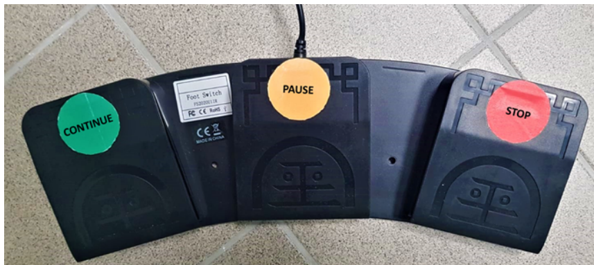
FIGURE 4.9: The pedal switch used to send "Continue", "Pause" or "Stop" signals to the system.
