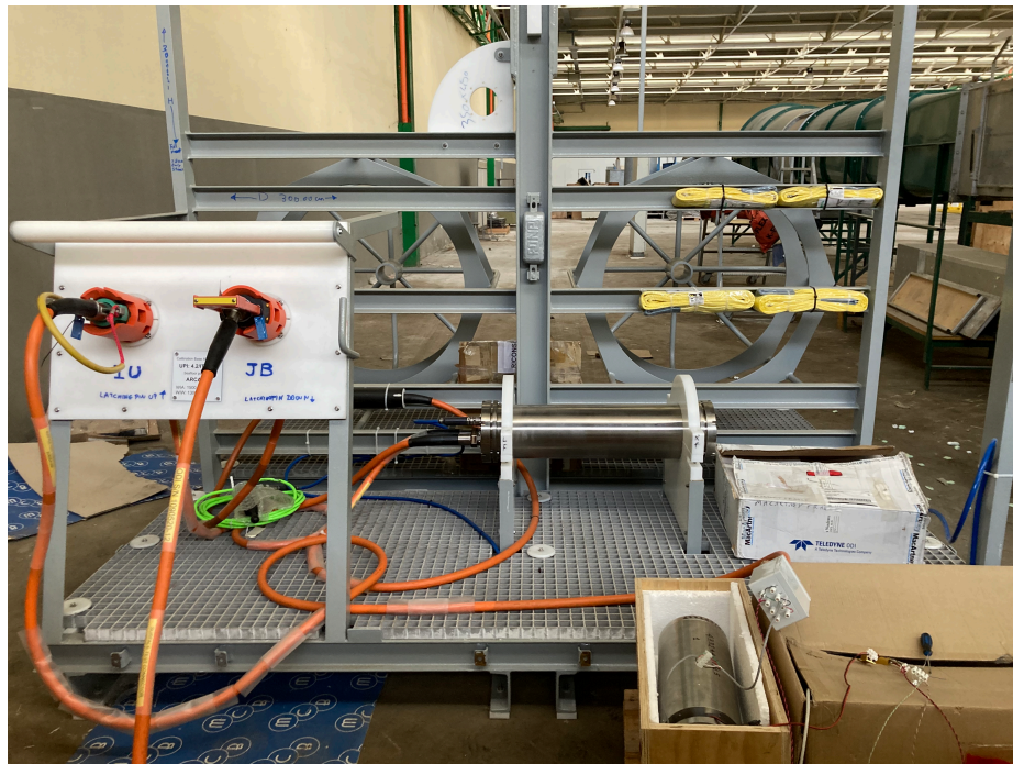
Figure 5.12: Tests of the Calibration Unit components. Top: open base module connected with the Data Acquisition test rack via a test cable (orange one). Hydrophone and beacon were connected via the GISMA ® connector and jumper cable (blue one). The Instrumentation Unit base container was connected via a 800 m Ethernet cable and power lines with a 20 Ohm resistor. Bottom: sealed base module linked to the front panel connector handled by the remote vehicle. The communication was established through the cable, made by Teledyne ODI ® , plugged to the front panel (connector on the right), with its test box connected to the Data Acquisition rack. The Instrumentation Unit base container was also connected with a cable with test box, and through 800 m of Ethernet cable.
