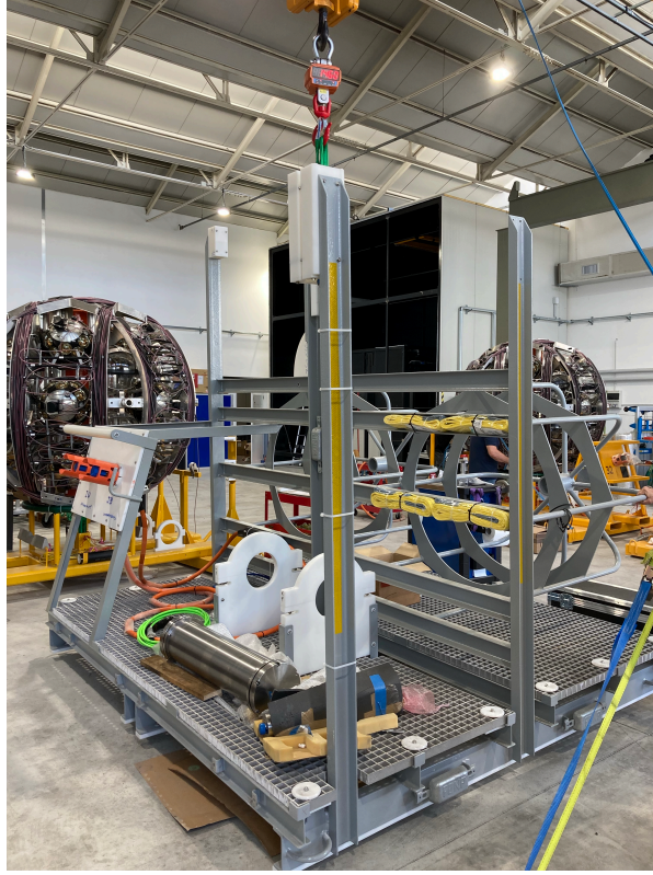
Figure 5.4: The Calibration Base during the weighting test at the Caserta facility. The base module, laid on the frame floor, the two orange jumper cables which connect it to the front panel, and the hydrophone (with the green cable) are visible.
