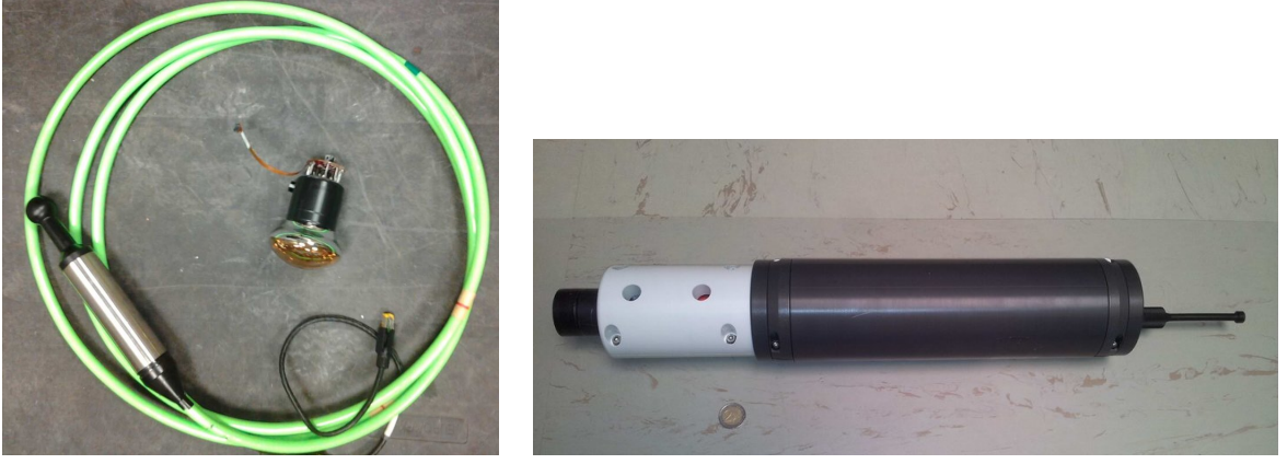
Figure 5.1: Left: the hydrophone used in KM3NeT, a Colmar ® DG1330. Right: the acoustic beacon used in KM3NeT, a MAB 100 from Mediterraneo Senales Maritimas ® .
