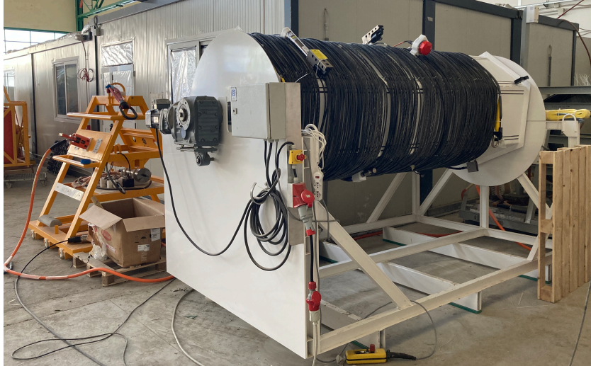
Figure 5.14: The spooler used for the deployment of the Instrumentation Unit. On its left, the Instrumentation Unit frame can be seen, connected with the 700 m cable to the Calibration Base (not visible) during the final functional test.
