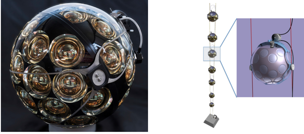
Figure 2.10: Left: an assembled Digital Optical Module. Right: schematic representation of a part of a Detection Unit.
