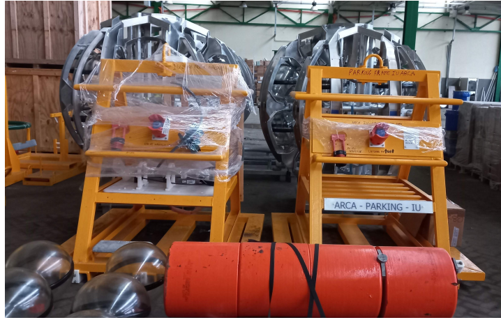
Figure 5.9: Instrumentation Unit recoverable frame (on the left) and the parking frame for the connector of the interlink with the Calibration Base.
