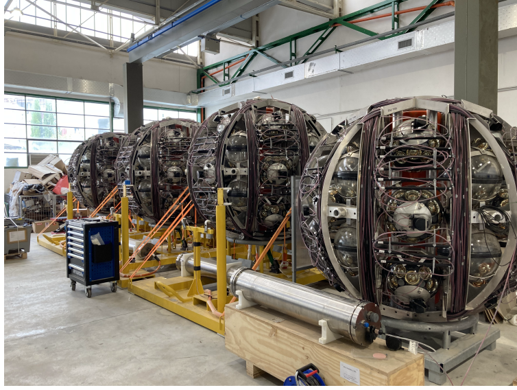
Figure 2.12: KM3NeT/ARCA Detection Units mounted on LOMs and ready to be deployed. The Base Module titanium cylinders (of the Standard White Rabbit architecture type) can be seen.
