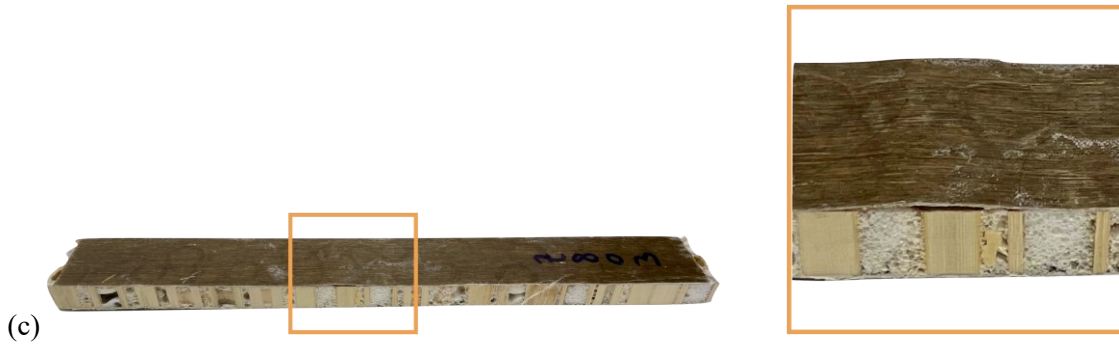
Figure 16. (a) Failure mode for unpolished lateral surface; (b) Failure mode for P120 polished lateral surface; (c) Failure mode for Z80 polished lateral surface.
