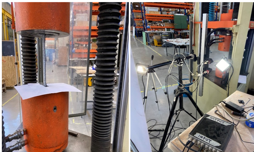
Figure 54. On the left, is the Galdabini Machine used for the tensile test. On the right, are the Digital Image Correlation instruments.
