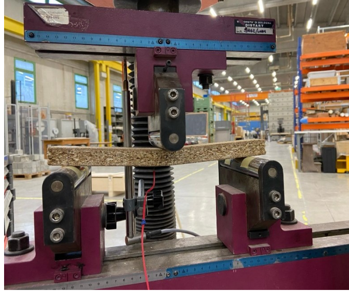
Figure 25. Three-point bending test on a sample of 300 x 50 x 22 mm.
