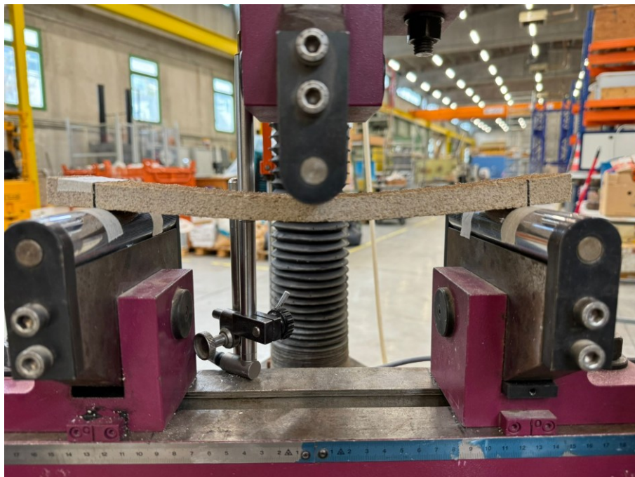
Figure 48. Setup of the three-point bending test
